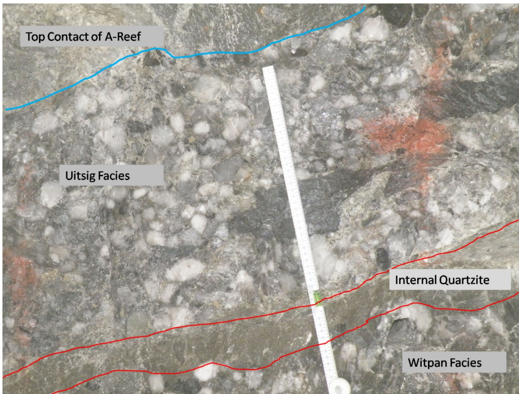
Figure 3-2: A Reef unit depicting a section of the top and bottom units and also showing the immature interbedded quartzwacke between these units (photograph was taken under ground by the author at Brand 1 Shaft where A Reef has been mined until 2010).
