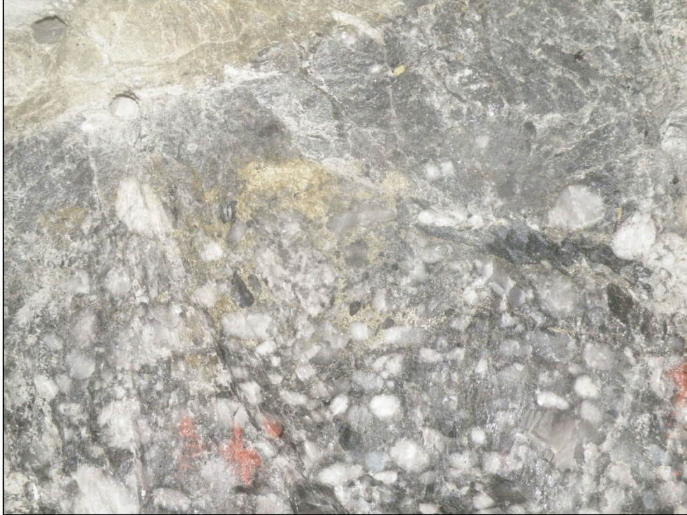
Figure 3-21: Sporadic pyrite concentration in the A Reef (photograph from underground visit to Brand 1 Shaft).
