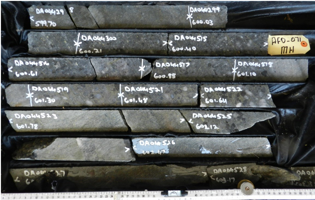
Figure 3-13: Example of Gmc facies, upward fining small pebbles and grits that occur as sheets along channel edges.
