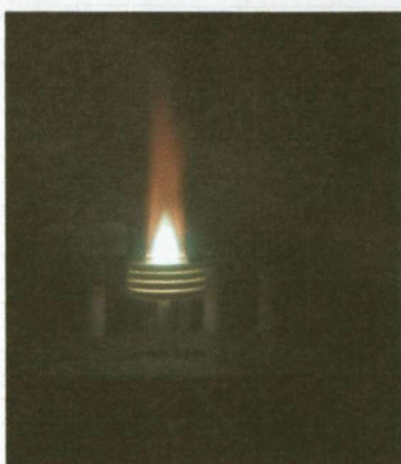
Figure 4.11: Plasma appearance in the presence of a sodium salts flux fusion solution.
