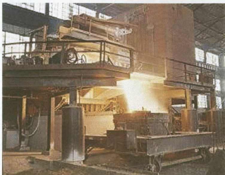
Figure 2.5: Production of ferro-niobium alloy in an electric arc furnace
