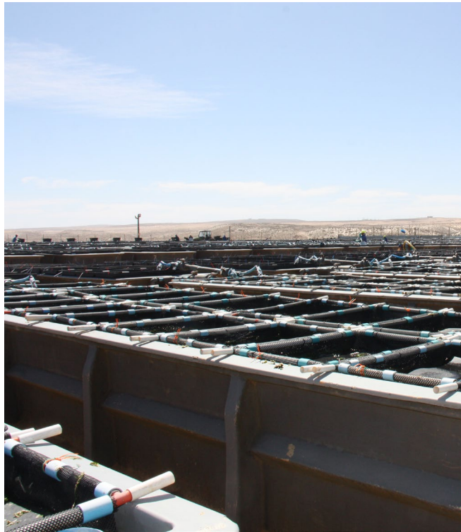
Figure 64. Abalone Raceway Tanks - existing grow-out tanks in Kleinsee for the growing of abalone (author, 2023)
