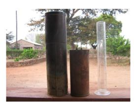
Figure 5.1: Standard rain gauge used in Zambia, left side is outer brass cylinder in the middle is the inner cylinder and on the right is the glass measuring cylinder to ensure accurate measurements.
