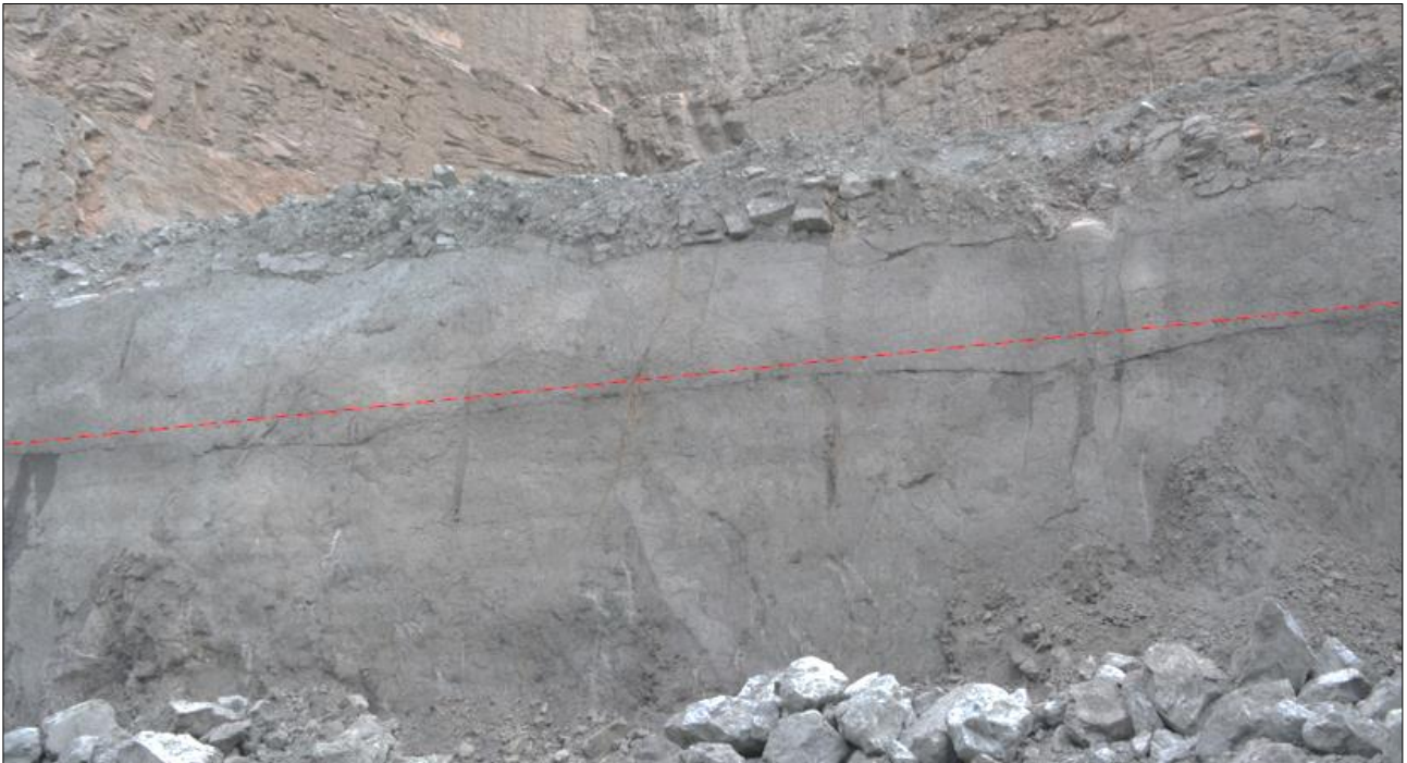
Figure 4-5 Basal zone, more competent basalt with some jointing.
