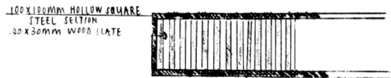
Figure 169: Ventilation structure (author,2023).
