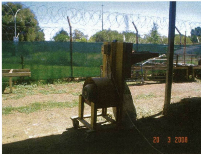
Figure 2.5 Small hammer mill used to coarsely ground the sun-dried Opuntia cladodes and lucerne hay.
