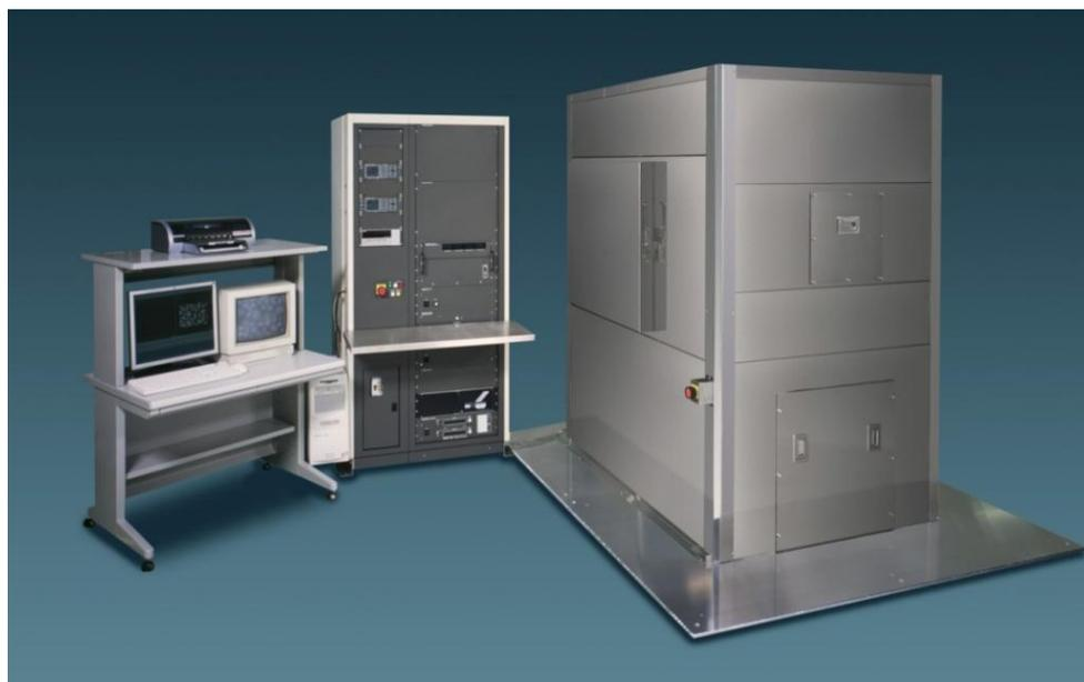
**Figure 7.7:** The PHI 700 Auger Nanoprobe used for obtaining depth profiles, elemental maps and SED images of the polycrystalline bcc Fe samples.
