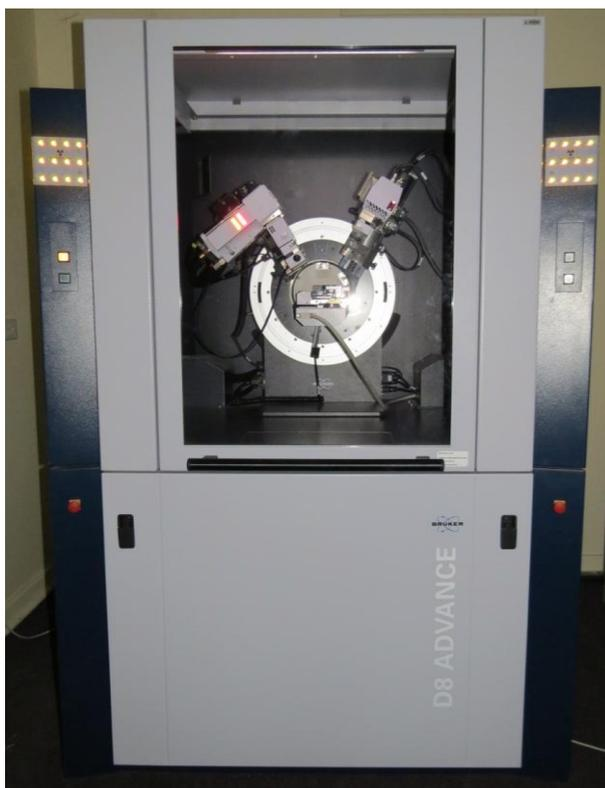
*Figure 7.2: The D8 ADVANCE X-Ray diffractometer used for the determination of the crystal orientations present in polycrystalline Fe samples.*
