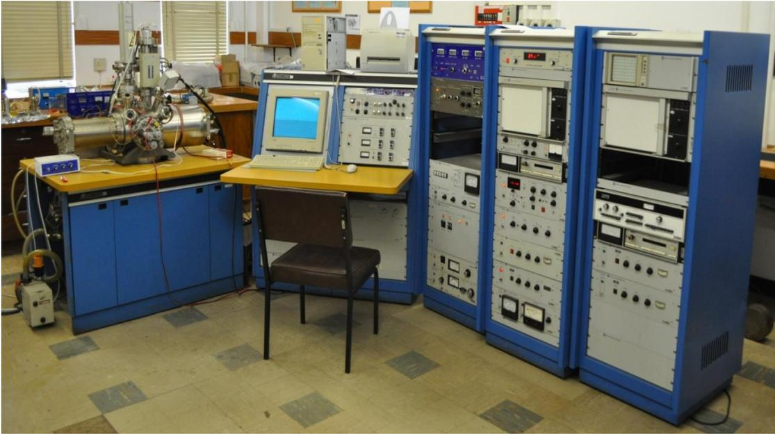
*Figure 7.6: The SAM 590 Auger system used in the study of non-metal impurity surface segregation in polycrystalline bcc Fe.*
