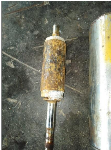
Figure 93 – Image showing precipitate build-up on the borehole water supply, from parts of the submersible pump.
