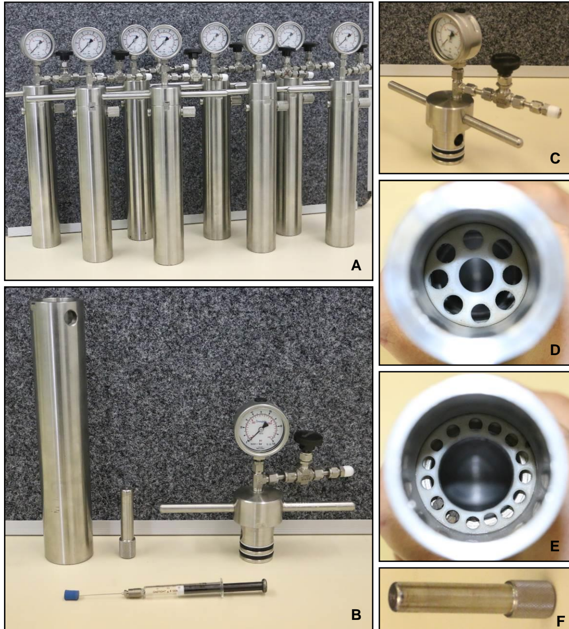
Figure 5.5: Images of (A) all the constructed syringe incubators, (B) the individual components of a syringe incubator, (C) the lid, (D) the 5 ml syringe ring, (E) the 25 ml syringe ring, and (F) the safety pin.
