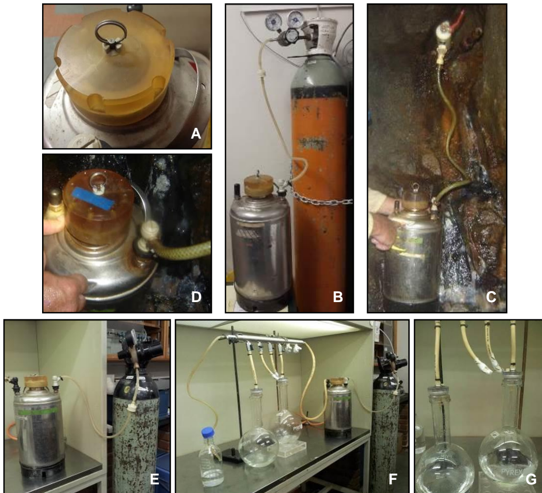
Figure 3.11: Methods used for (A) sterilizing the canister with the outlet valve opened, (B) flushing the canister, (C and D) collecting fissure water on-site, and (E-G) filtering water from the canister.
