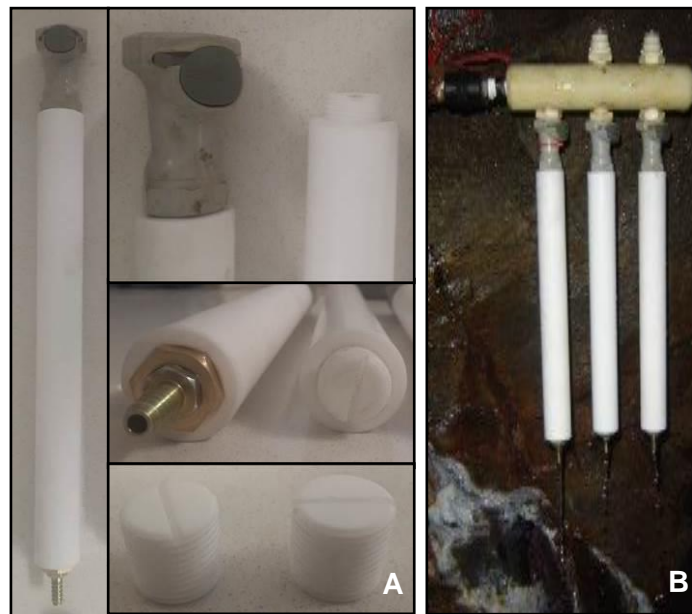
Figure 3.16: (A) The custom made PVC cartridges with its fitting and caps and (B) the cartridges directly connected to the sampling manifold on the borehole.
