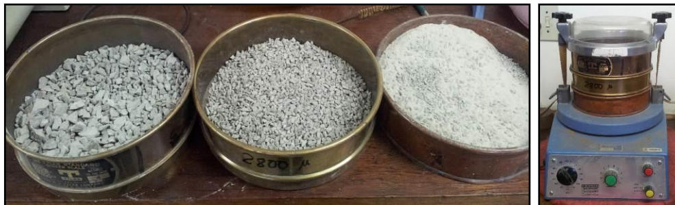
Figure 3.10: Separation of the crushed rock using a 2.8 mm and a 4.7 mm strainer.
