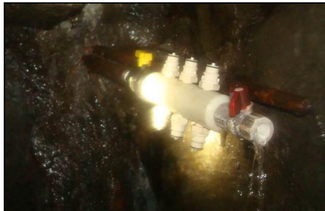
Figure 3.5: The organic-free manifold used for sampling, connected to the casing inside the borehole.
