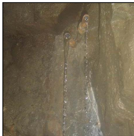
Figure 3.4: The encased borehole, intersecting the Karoo sandstone fissure water, which was used for sampling in the Star Diamonds mine.
