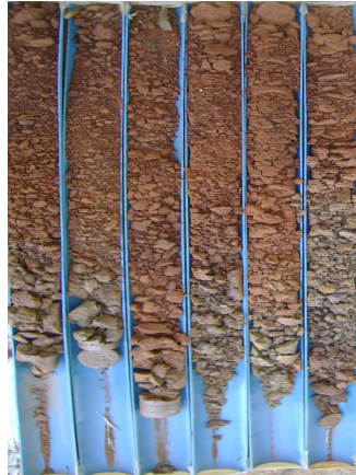
Figure 5.3 Sampled soil cores taken with the hydraulic auger.
