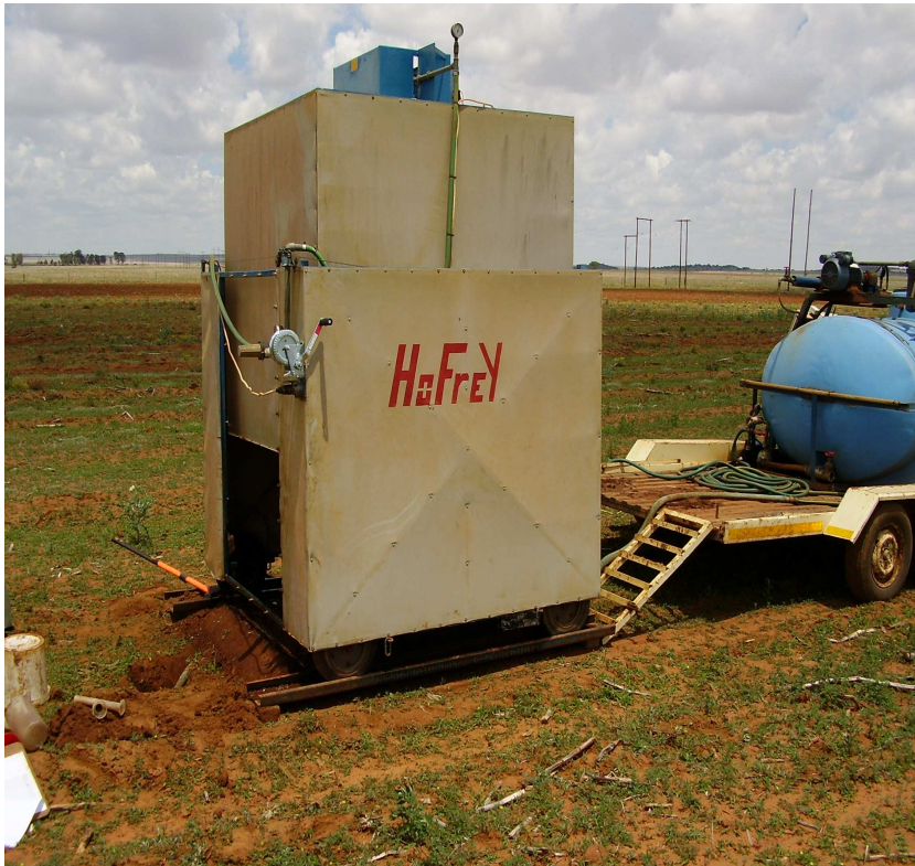
Figure 6.2 The HoFrey rainfall simulator, comprising of the sprinkler chamber, pressure adjustable pump unit, tri-osmoses filter and tank mounted on the trailer. The runoff-frame and gutter were installed under the spraying chamber that was levelled on two wheel tracts.
