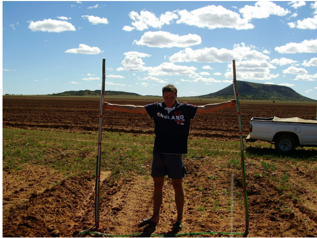
Figure 6.4 Handmade elevation measuring device, used to measure the slope of the runoff strips over a fix distance of two meters.
