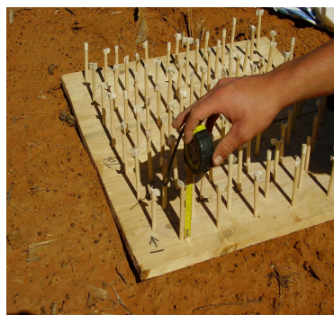
Figure 6.5 Handmade surface roughness measuring device, used to measure the roughness index of the 75 plots.
