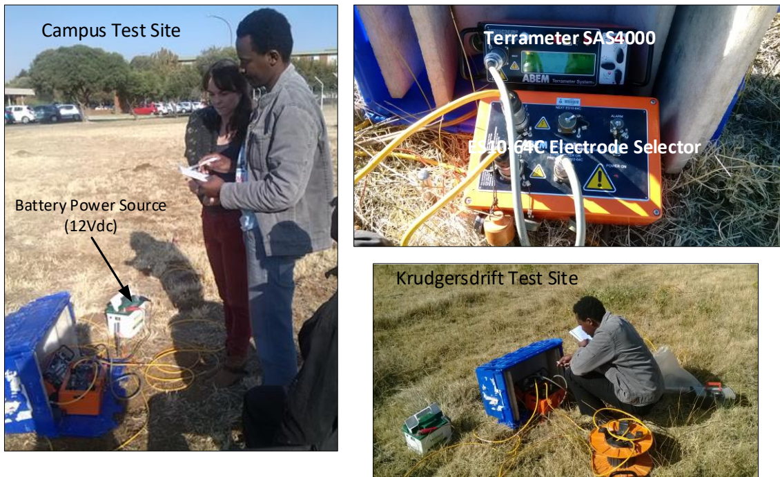
Figure 4.5: Photographs of resistivity survey at Campus and Krugersdrift Test Sites
