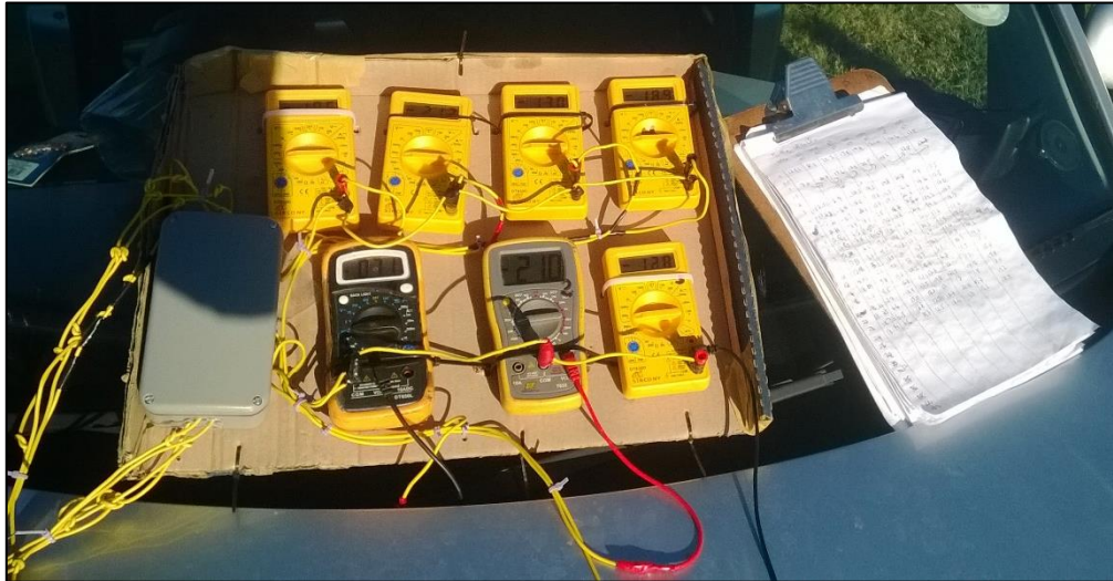
Figure 4.6: Voltmeters used to measure streaming potentials at each electrode station.
