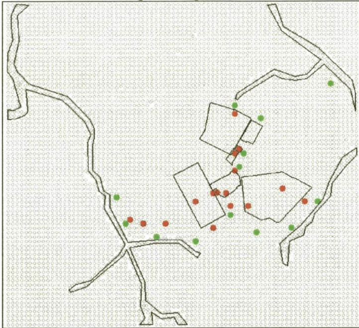
Figure 60: Positions of pollution sources (red) and observation points (green) for stochastic risk assessment
