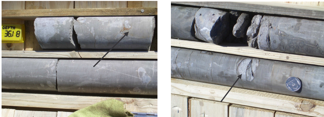
Figure 6-74: Enclaves within the mudstone layer providing preferential flow paths through their boundaries.
