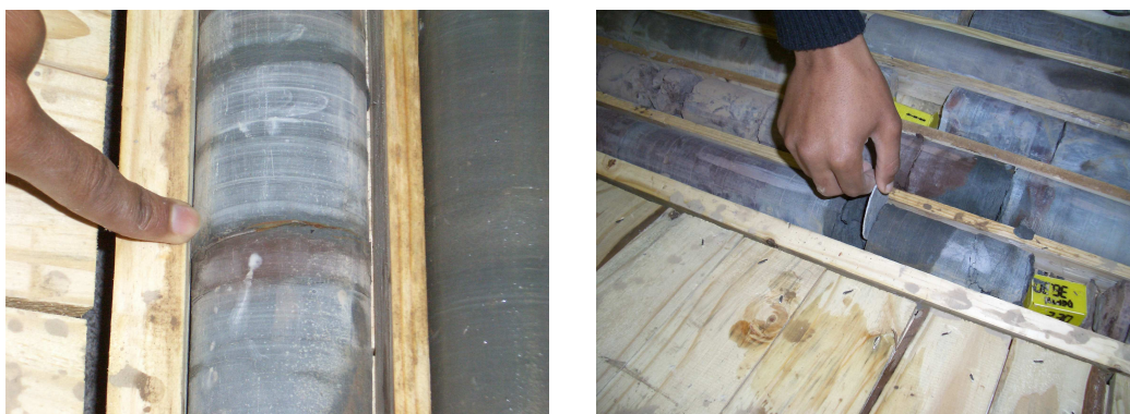
(A) Fracture partially filled with calcite vein
