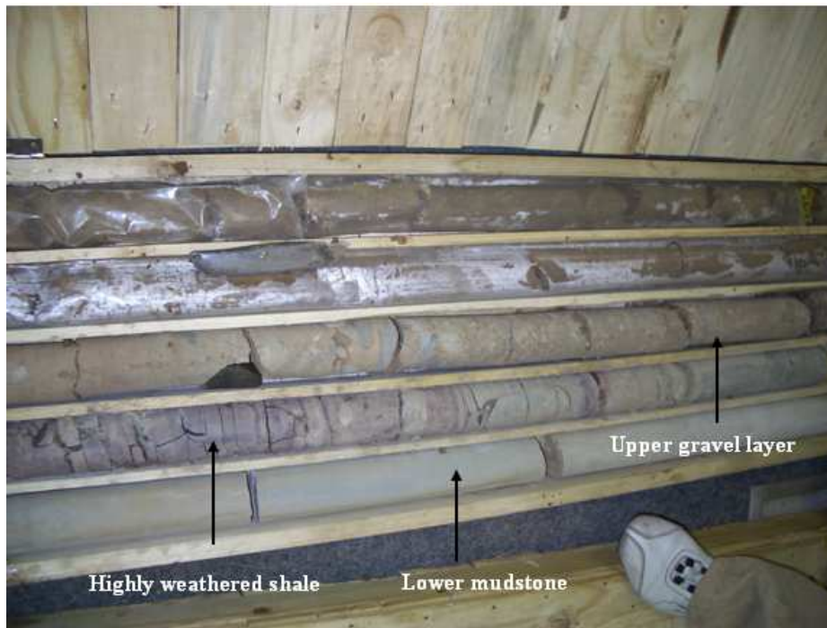
Figure 6-70: Highly weathered shale below the unconsolidated section in EC1.
