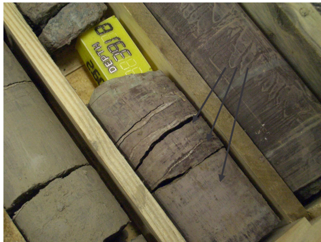
(g) Fracture zone filled with calcite veins
