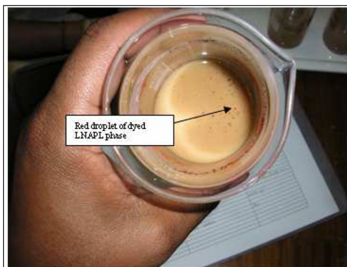
Figure 6-16: Detection of LNAPL droplet using the water-soil shake test with Sudan IV dye.
