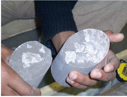
(c) Plan view of a fracture filled with calcite vein (vein broken during drilling)
