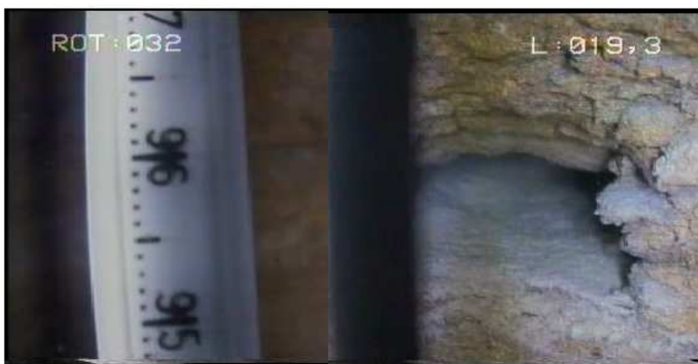
Figure 6-94: Video camera of Borehole D3 with accurate depth measurement and aperture of the fracture.
