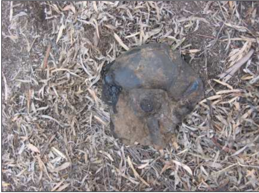
Figure 7-1: Example of excavated container with organic contaminants in a test pit at Test Site 1.
