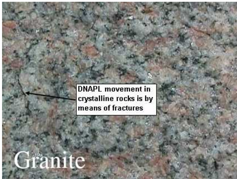
Figure 4-2: A granite sample with fracture but no significant void porosity. Flow is entirely controlled by the fracture orientation and properties of the DNAPL.
