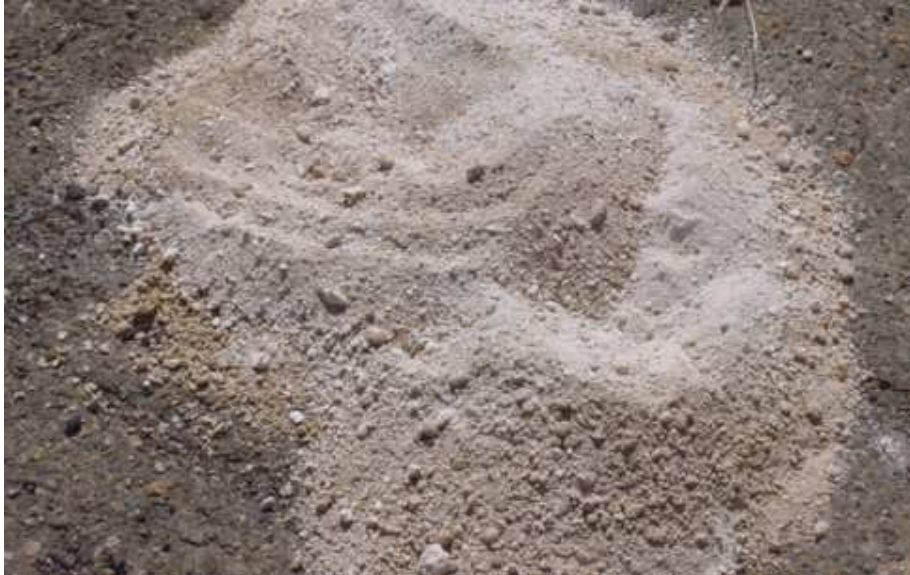
Figure 6-68: Calcrete at a depth of 10 m in Borehole GB2.
