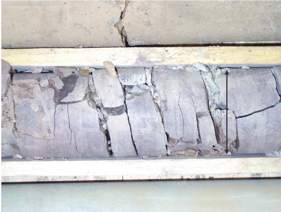
Figure 6-71: A closer look of the weathered shale in EC1.
