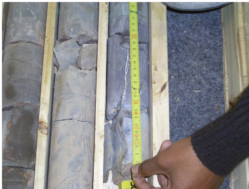
(e) Partially filled vertical fracture
