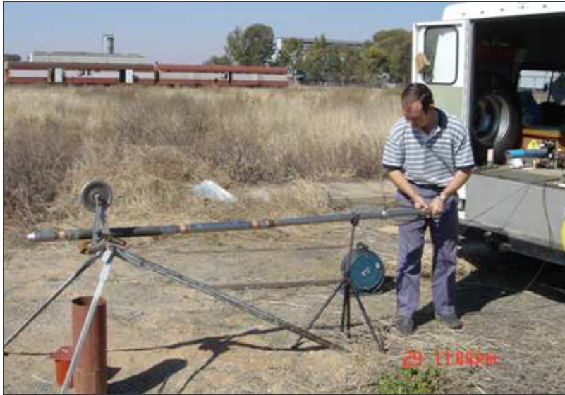
Figure 7-3: Geophysical logging of boreholes at research site - Test Site 1.
