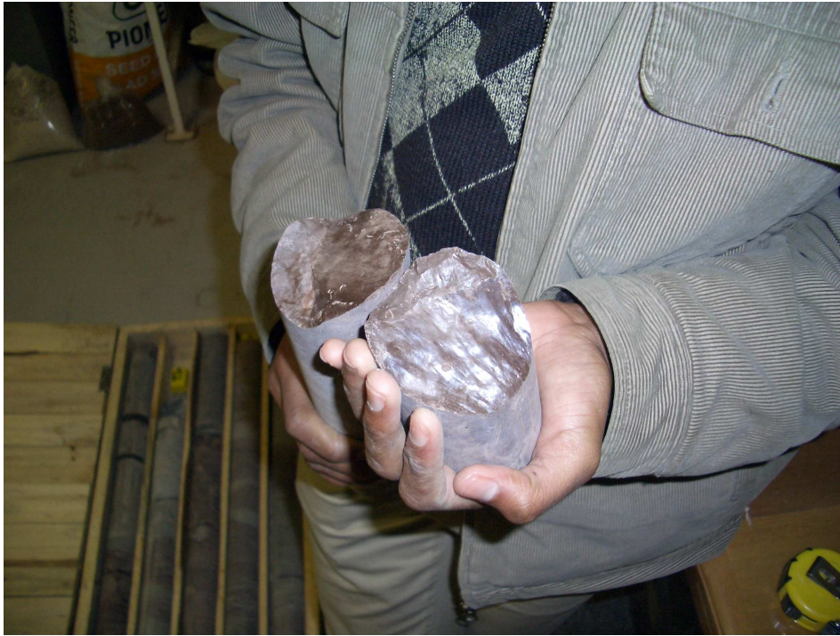
Figure 6-76: Slickensides showing shiny and grooved surface.
