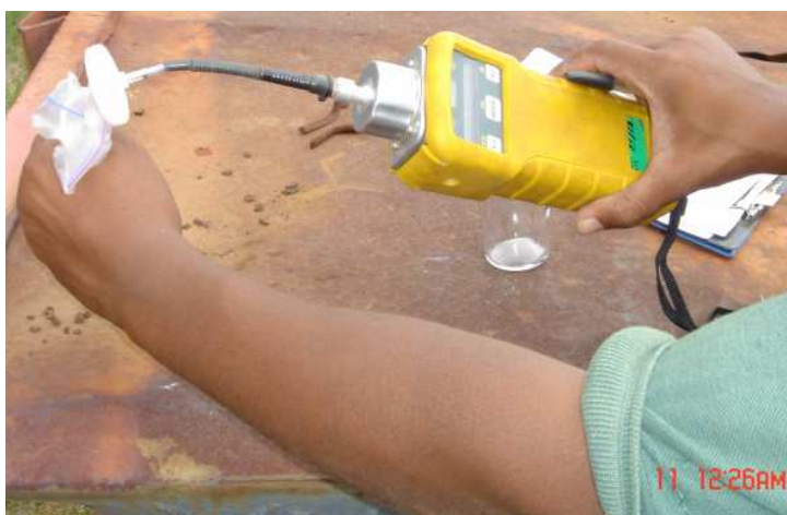
Figure 6-35: Hand-held PID reading VOCs of soil gas from a plastic container.
