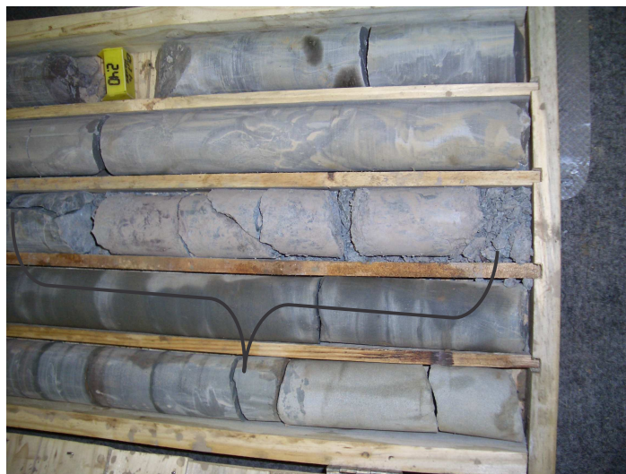
(C) Fracture zone around 41 m in GC1
