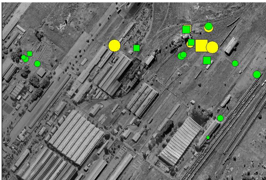
Figure 6-40: EC (mS/m) distribution of boreholes (circles) and piezometers (squares) on test site.
