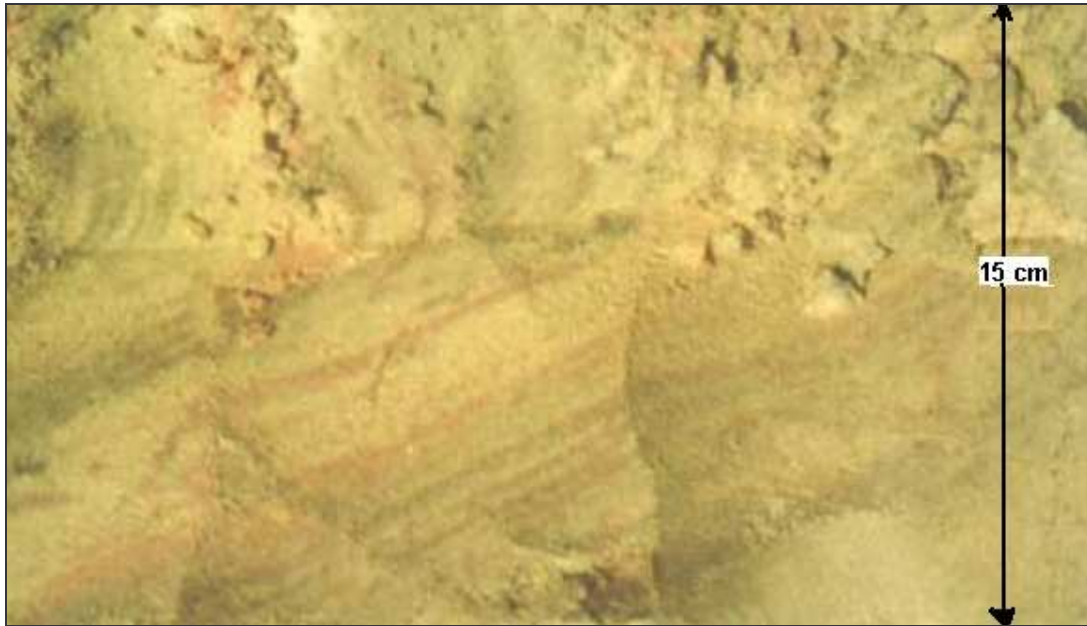
Figure 3-2: DNAPL migration pathways in unsaturated sands. DNAPL presence shows red due to SUDAN IV dye. Bedding dips 30° below horizontal (Poulsen and Kueper, 1992).
