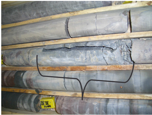
(A) Vertical fracture around 36 m in EC1
