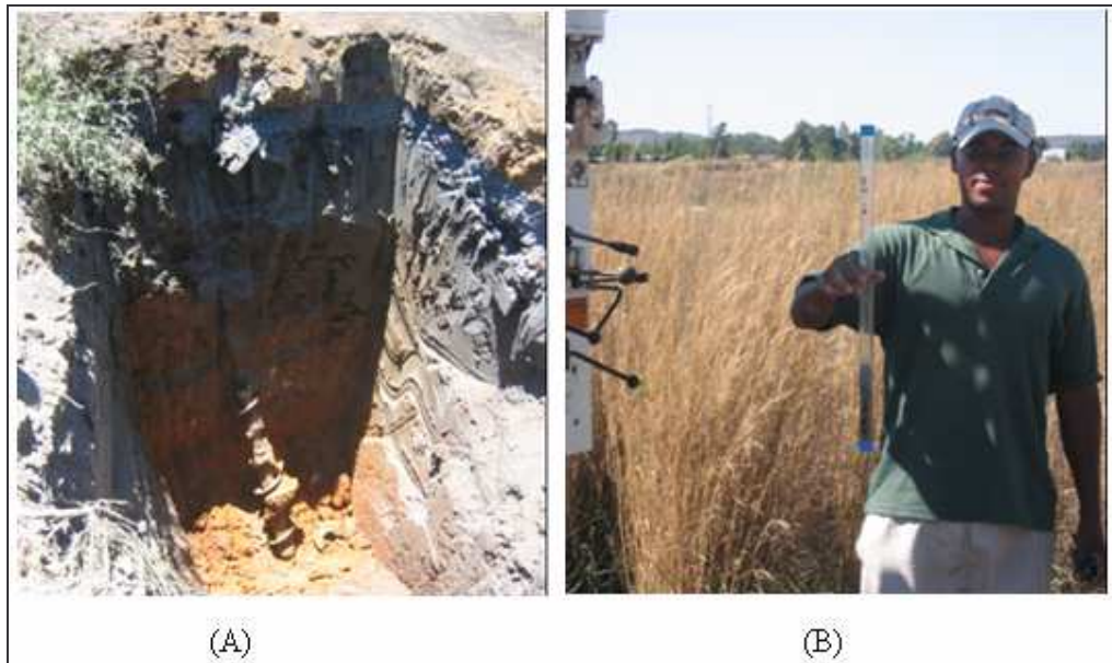
Figure 6-28: Auger drilling: (A) Hollow-stems stuck in the clay layer during auger drilling, (B) In-situ soil samples from direct push drilling.
