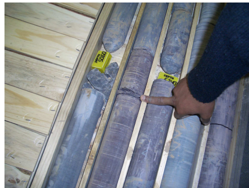
(B) Horizontal fracture around 51 m in EC1
