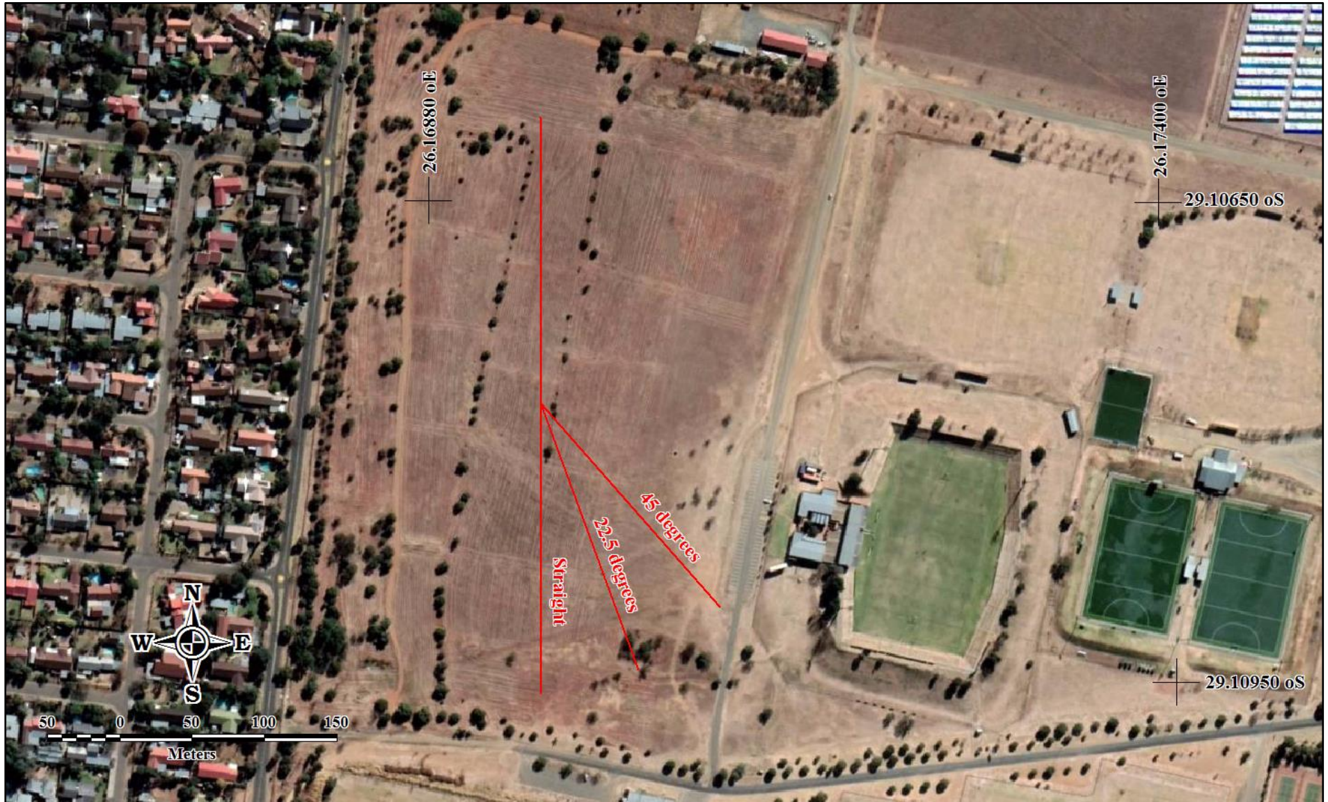
Figure 5.4. The geometry of the ERT survey on the UFS Campus
