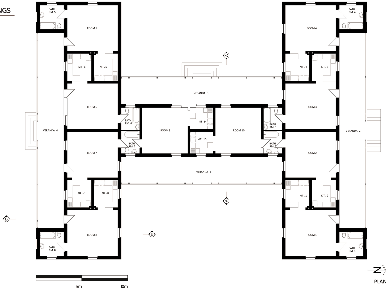
Fig. 14 Reproduced Ground Floor Plan of the 10-Mann-Haus with its current layout as part of the documentation process to have digital sets of drawings of historical buildings. (NUST, Department of Architecture (2017) Ground Floor Plan , 1:100. [Print] Held at: Windhoek: Namibia University of Science and Technology: Department of Architecture)
