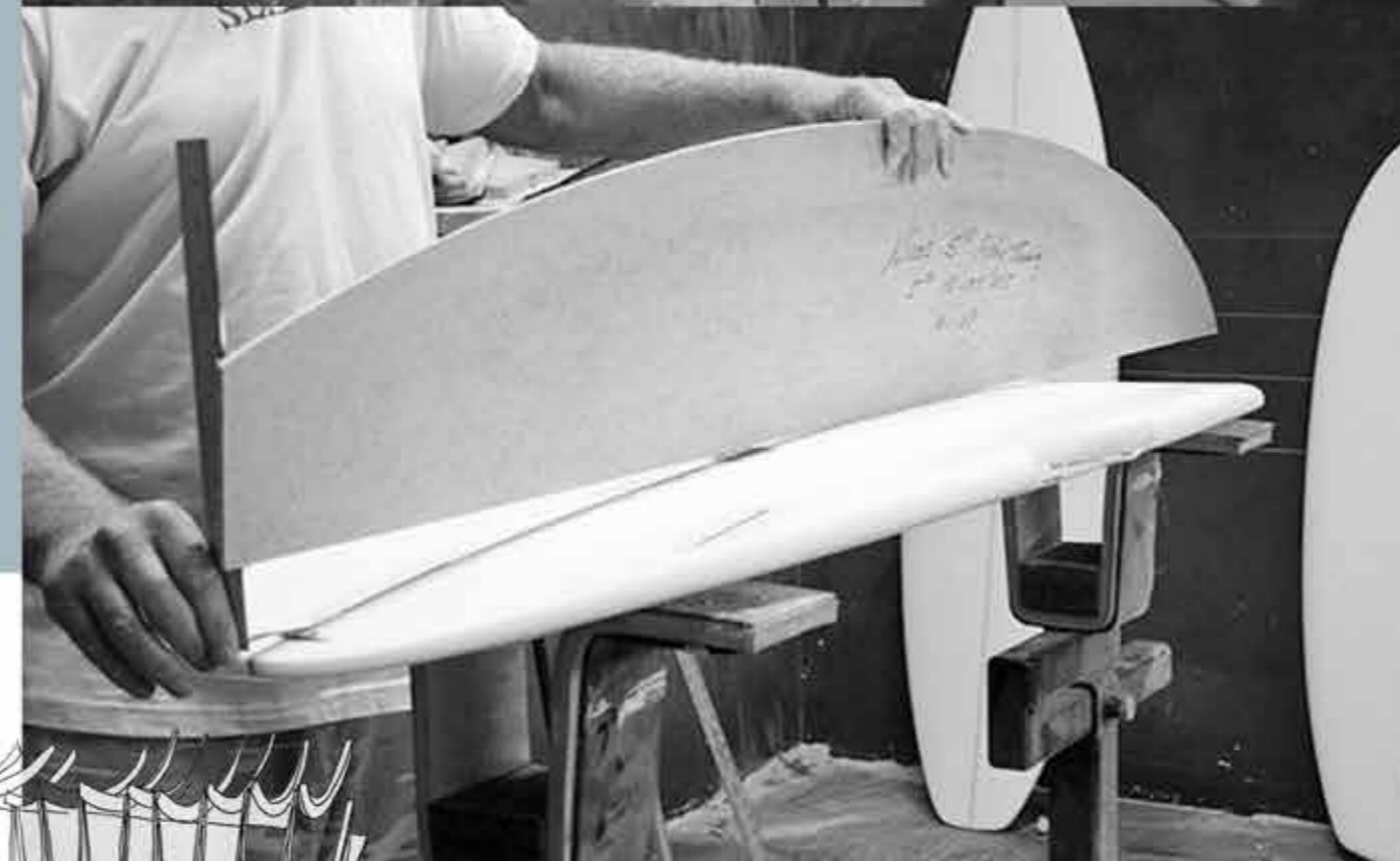
Figure 151. The shaper measuring the rocker, (Understand The Surfboard's Rocker - Surf Equipment Tips, 2020).
