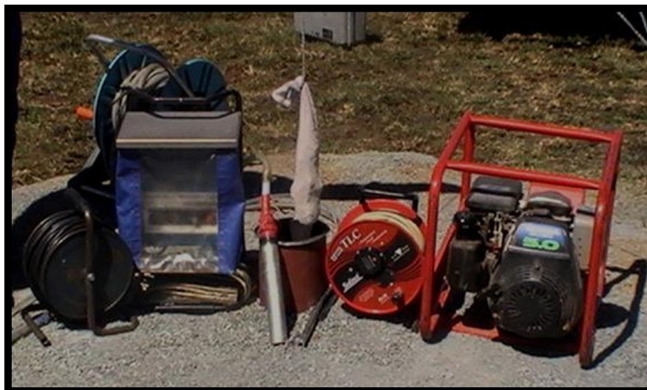
Figure 6-8 Equipment for conducting a transient state FEC-based dilution test
