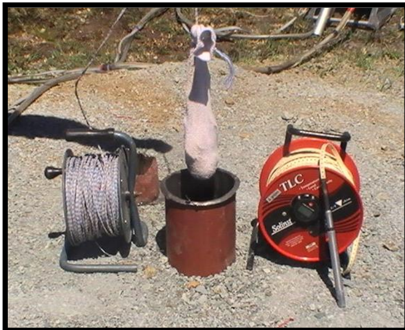
Figure 6-7 Equipment for conducting a transient state FEC-based dilution test
