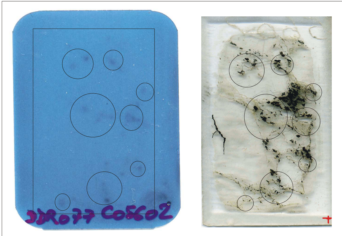
Fig.3-7: Image of the radioactive minerals on photographic film with the thin section, autoradiography method (Rogers 1979) on sample DDR 077 CO 5602
