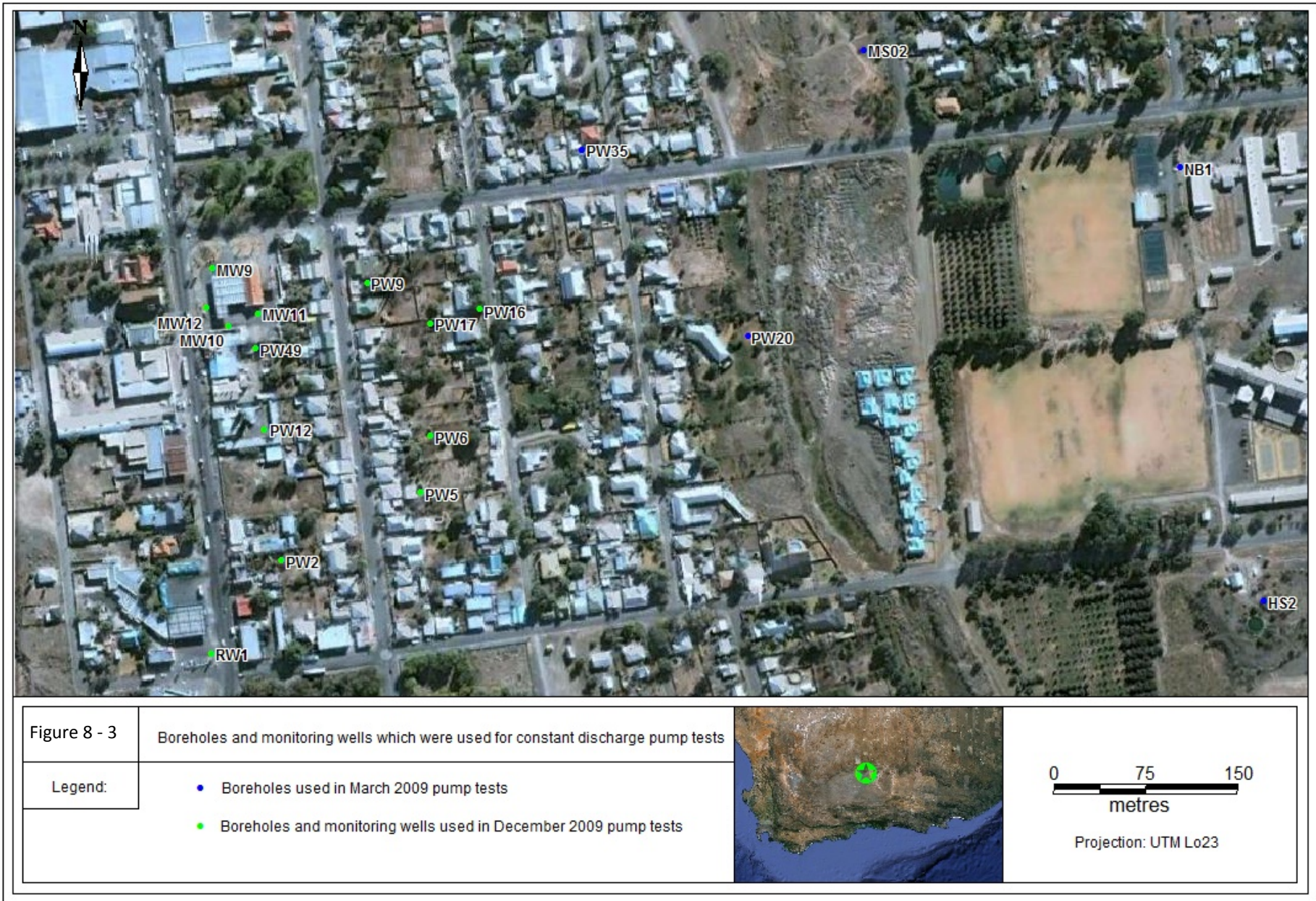
Figure 8-3: Site layout of boreholes and monitoring wells used in constant rate discharge test.
