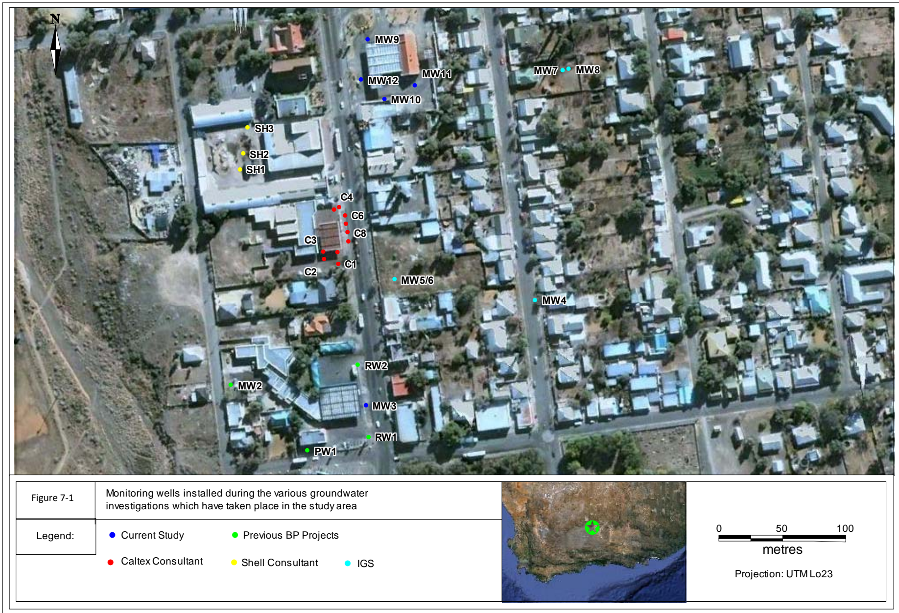
Figure 7-1 Monitoring wells installed during the various groundwater investigations which have taken place over the years
