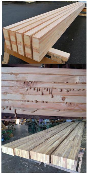
Figure 113: The Procces of laminating a wood beam
