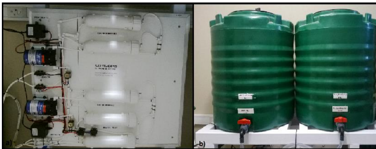
Figure 5.6: The process of reverse osmosis (a) and water storage facility (b).
