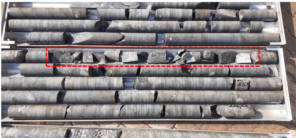
Figure 4.10 A typical example of a weathered-fractured zone in dolomite (marked in red). This picture was taken from borehole BHW 289 during core logging
