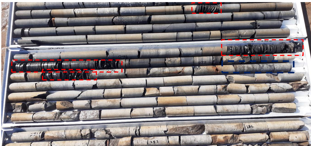
Figure 4.37 Picture showing dolomite core logs with some weathered shale lenses (marked in red)
