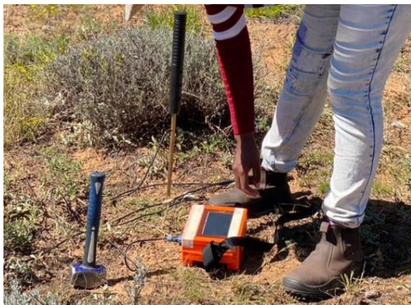
Figure 3.1 The ADMT 300s Electrical Groundwater Detector tool.
