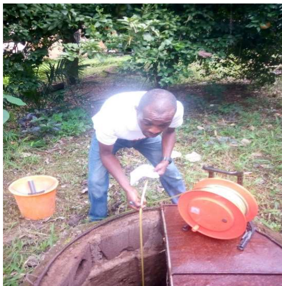
(a) Showing the use of an electrical water level probe
