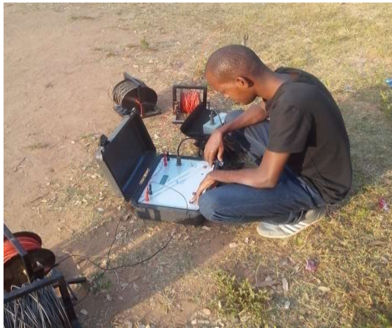
Figure 3.5 Collecting vertical electrical soundings data in the study area using Schlumberger array
