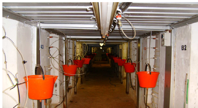
Figure 2.2 Underground chamber of the lysimeter unit showing that each lysimeter has a manometer through which the height of the water table was regulated by recharging from a bucket.
