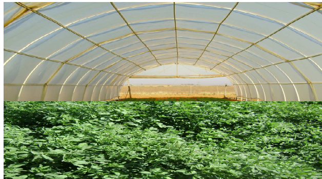
Figure 5.1 Lucerne under the movable shelter (30 m long, 10 m wide and 4 m high), covering the lysimeter unit to prevent the influence of rain.
