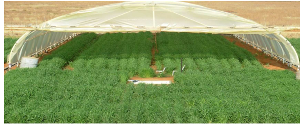
Figure 4.1 Wheat under the movable shelter (30 m long, 10 m wide and 4 m high), covering the lysimeter unit to prevent the influence of rain.
