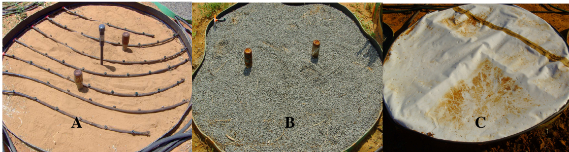
Figure 3.1 Illustration of the surface treatments on the Clovelly soil of experiment one, viz. (A) the bare soil surface for the reference evaporation, (B) a 50 mm thick gravel mulch (dolerite with a mesh size of 10 mm) and (C) a white plastic for 100% soil surface cover, all equipped with neutron probe access tubes and a surface drip irrigation system. The same layout was repeated for Bainvlei soil.
