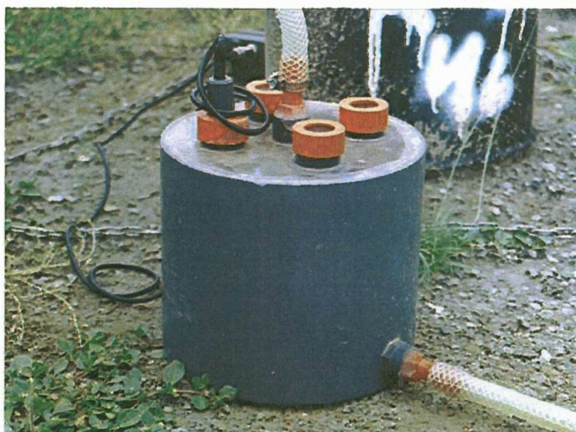
Figure 5-7 Through-flow cell for measurement tracer concentration and physico-chemical properties of the water using electrodes (e.g. EC, pH, Ion sensitive Sensor)
