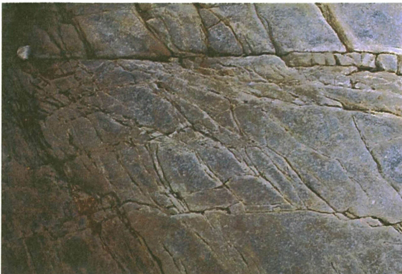
Picture 1 Natural fracture network in a sandstone outcrop (Table Mountain Group, Hermanus)
