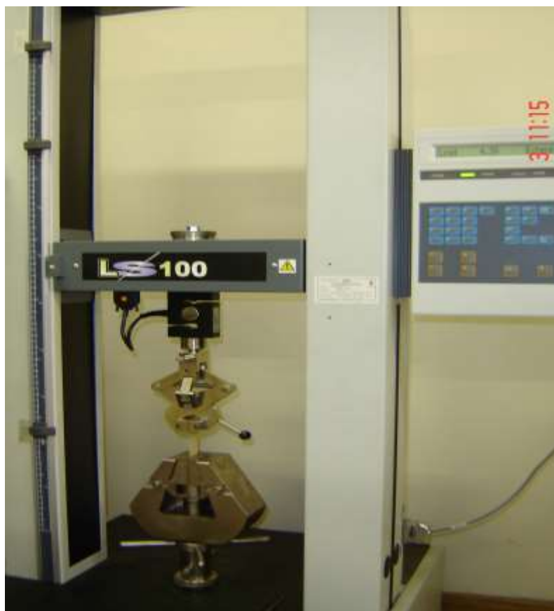
Figure 6 The Lloyds LS100 twin column tensile strength tester used for tensile strength testing of different pericardial samples
