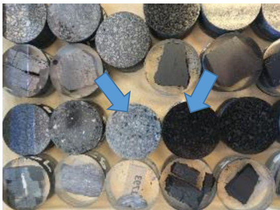
Figure 5-2 : Epoxy-mounted lump and particulate block, 300 mm diameter. The left arrow indicates the ash sample obtained immediately below the heat affected sandstone (S9); the right arrow indicates the coal sample taken immediately below the ash layer (S10).
