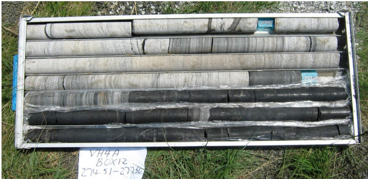
Figure 4-5 Gus seam section of the drill core of G1VH4, the coal seam starts at 277.81 mbg (black core section)
