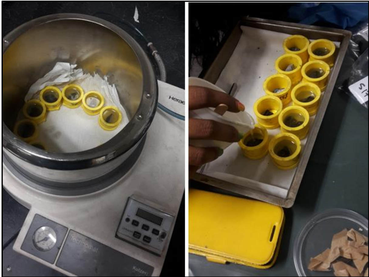
Figure 4-4 Sample preparation for QEMSCAN analysis, block samples are put in 30 mm diameter sample holders and carnauba wax is added (right). The mixed sample was placed in a pressure vessel set at 2 bars for 5 to 12 hours (left)
