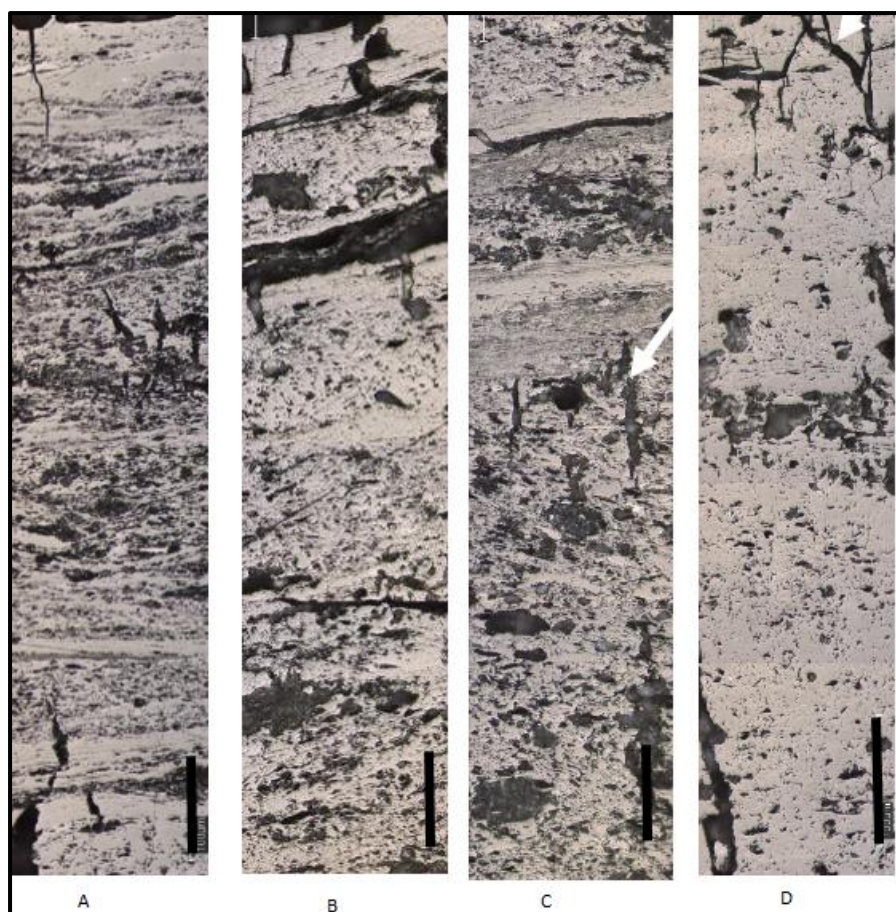
Figure 5-5 Mosaic images of lump VH3 core samples. A) S10 / 1794, note the devolatilisation pores in the vitrinite band towards the top of the image; B) S11 / 1797, note the large cracks in the vitrinite band towards the top of the image; C) S14 / 17103, note the perpendicular, epigenetic carbonate cleats; D) S17 / 17108, note the cracked nature of the vitrinite band towards the top of the image; cross linking of the cracks is evident. (reflected light, x50 oil objective, scale bar is 100 microns).
