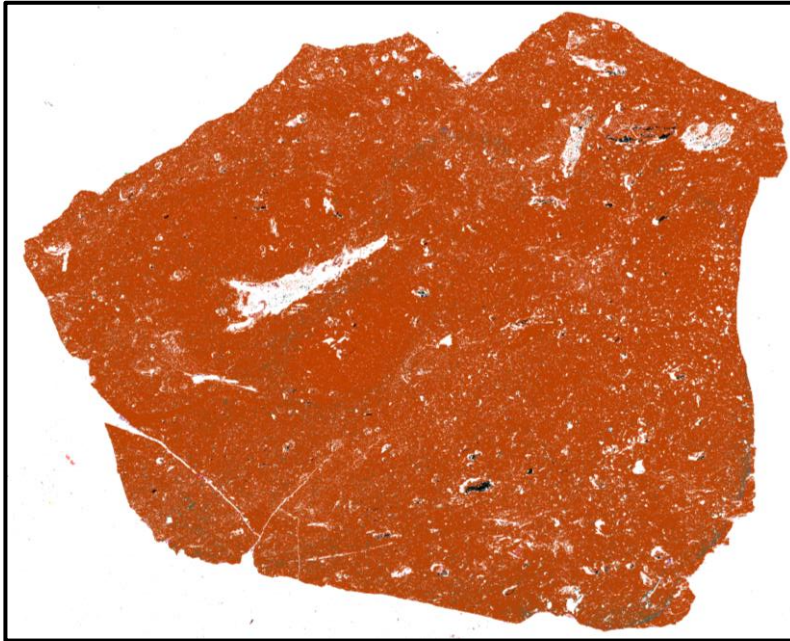
Figure 4-27 QEMSCAN image of sample M-ash, which is almost completely composed of metakaolinite (brown).
