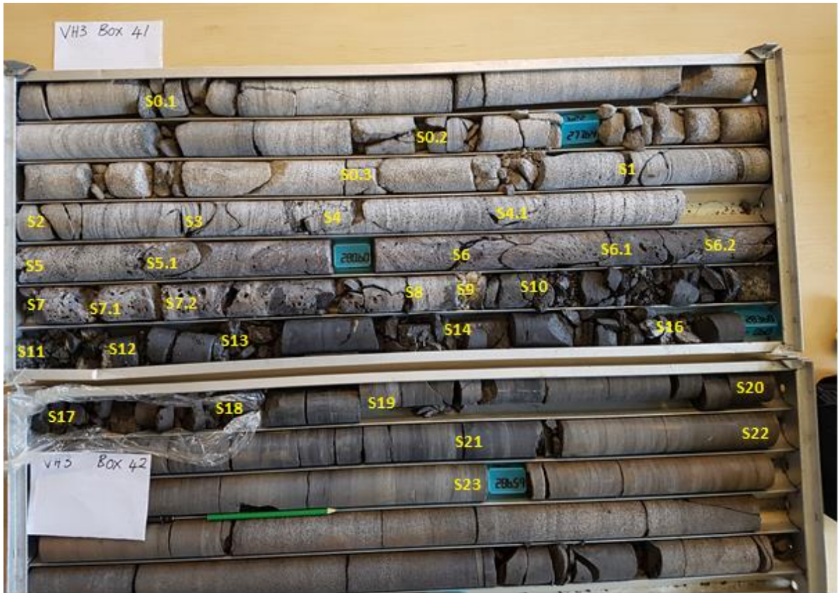
Figure 4-2 Core sampling of VH3, the same sample numbers will be used throughout this document
