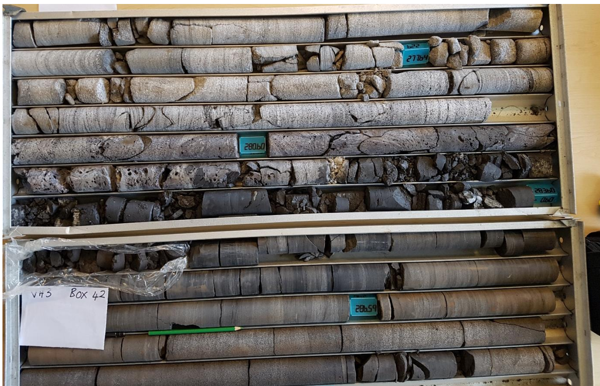
Figure 4-7 Gus seam section of the drill core of G1VH3, the ash layer at 281.7 mbg is the bottommost part of the overburden and represents the overburden-char contact.
