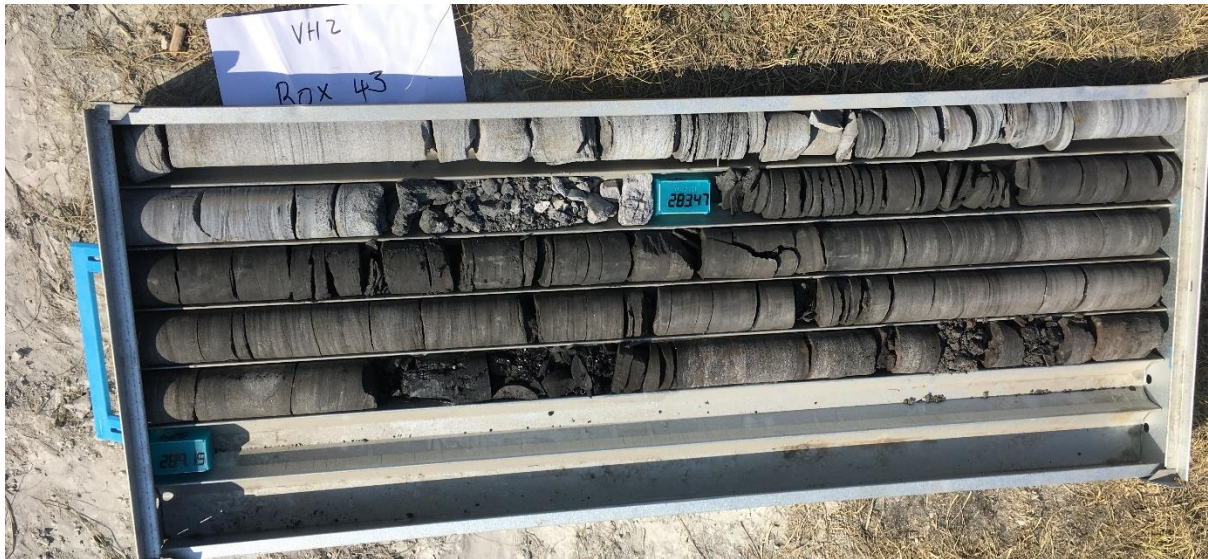
Figure 4-6 Gus seam section of the drill core of G1VH2, the coal seam not recovered and bottom of overburden shown by the 283.47 mbg (blue marker). Carbonaceous shale (coal seam floor) begins after the blue marker
