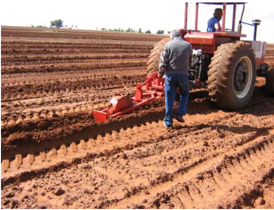
Figure 1.5 The basin plough creating 10 cm deep x 1 m wide basins along the contour ridges.
