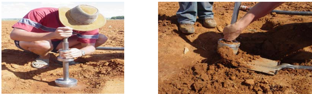
Figure 3.10 Illustrating the sampling of the soil for bulk density determination (a) The core is inserted into the soil with a sliding hammer and (b) recovered without disturbing the soil inside the cylinder.
