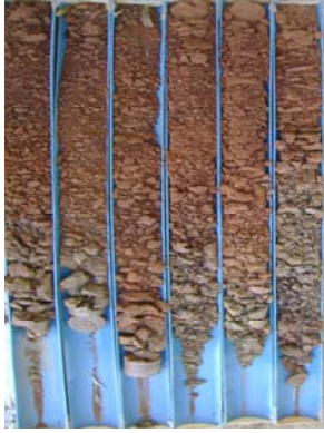
Figure 2.8 Soil cores drawn using the hydraulic core sampler.
