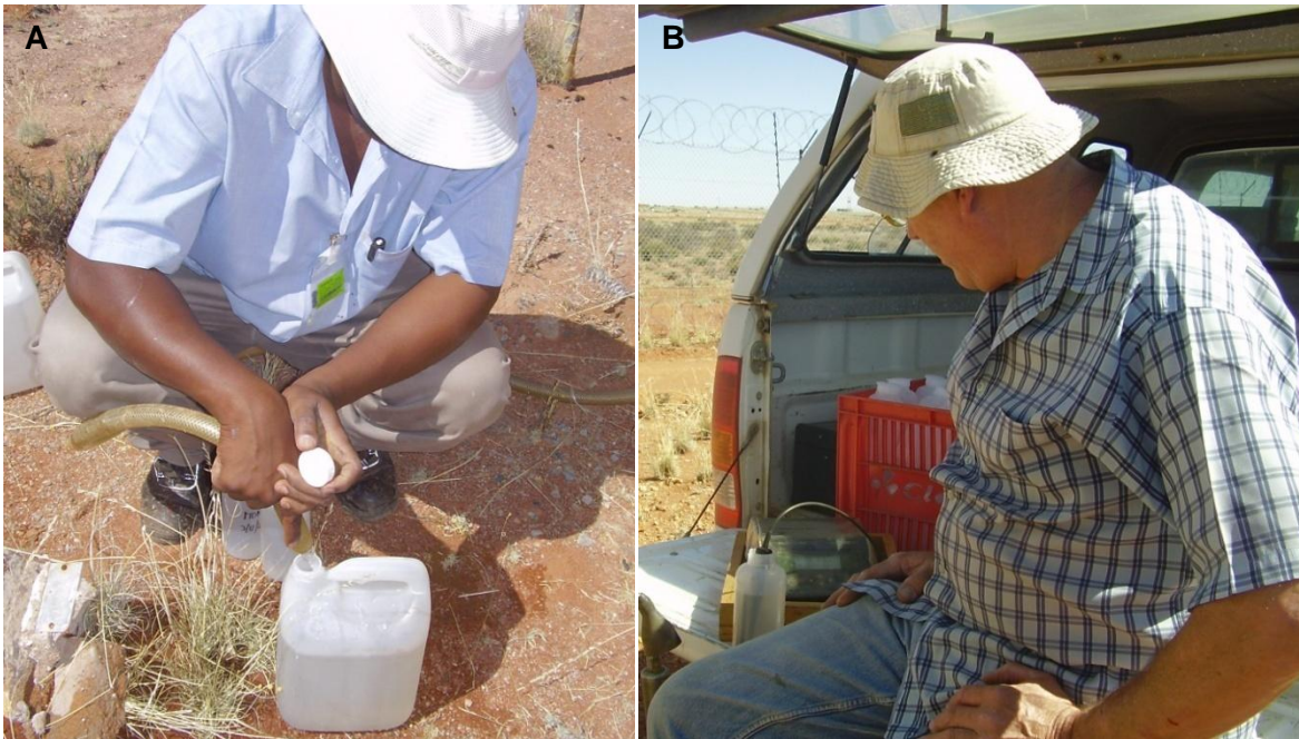
Figure 5.2A: Sample holders are filled with water. B: On site measurement of temperature, electrical conductivity, Eh and pH.
