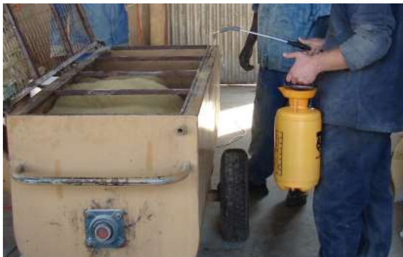
Plate 3.4 Blending of supplementary lipid source with the basal diet using a paddle-type feed mixer
