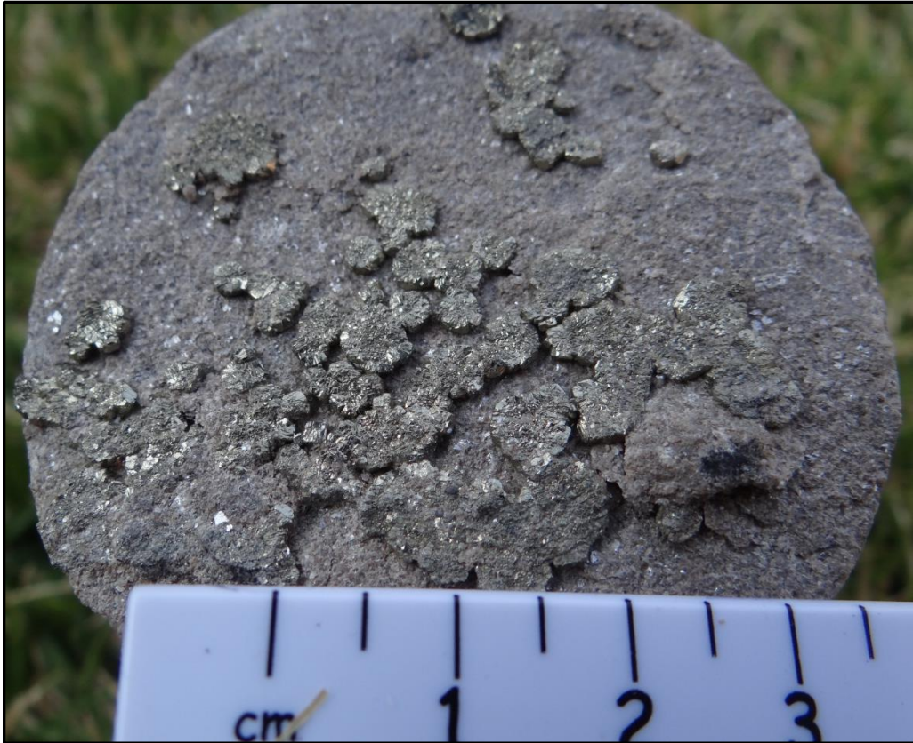
Figure 128: Pyrite in sandstone layers (135-138m depth).
