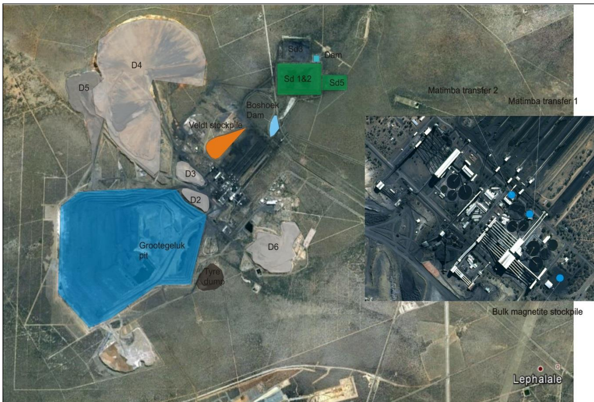
Figure 7: The Grootegeluk pit (blue), processing plant (right insert), discard dumps (D2-D6) and slime dams (Sd1, 2 and 5) (Google map & Mac Donald 2015).
