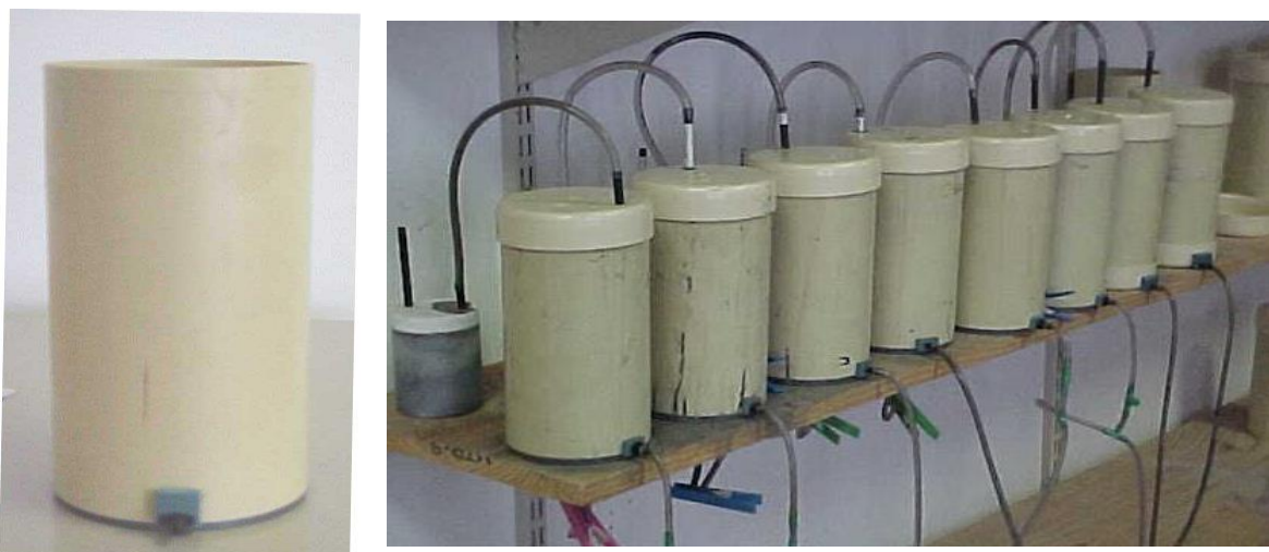
Figure 40: An IGS humidity cell (left) and an array of cells set up at the IGS (right).
