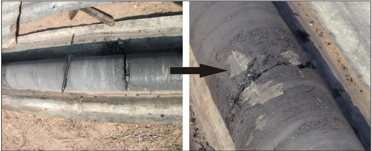
Figure 32: Core sample from exploration borehole near the GCM, with large pyrite hosted within the coal.
