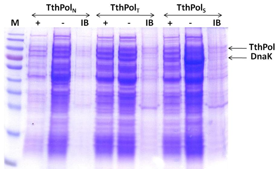
Figure 3.4. Expression profiles of recombinant *Tth*Pol in *E. coli*, as shown by SDS-PAGE. Lanes showing IPTG induction (+) and no IPTG induction (-) are shown along the insoluble fraction (IB) after 6 hours. M is the molecular weight marker used for all protein gels. In all profiles, the decrease in protein content can be observed after induction with IPTG as a result of increasing metabolic load.
