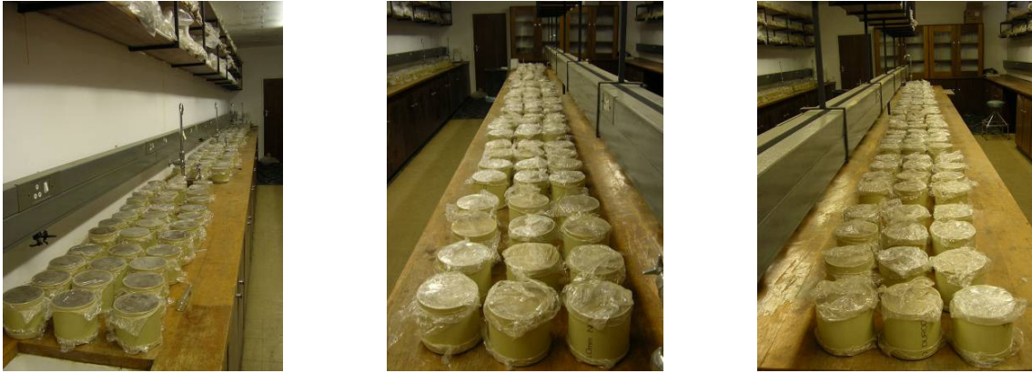
Figure 6.3 The 408 soil cores stored at a constant temperature (23°C).
