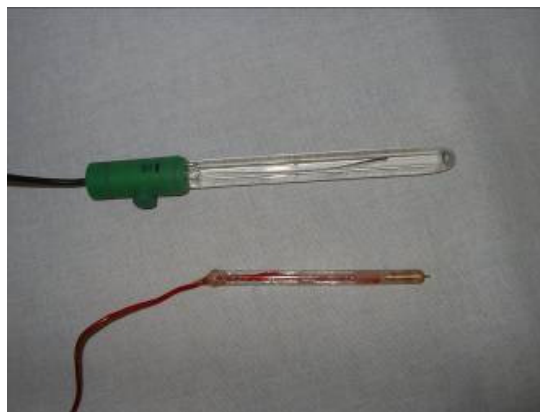
Figure 6.1 Glass Ag/AgCl reference electrode with accompanying Pt redox electrode.
