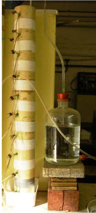
Figure 5.2 Soil column constructed from ten 0.1 m segments with a permanent water table at 0.3 m from the base of the column using a Marriot bottle (Marriot bottle not visible in picture).
