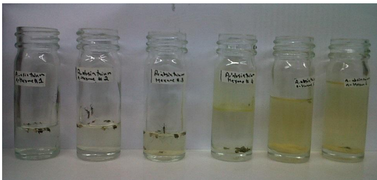
Figure 4.4 The larvicidal and pupicidal bioassays experimental setup with graded extract concentrations for Culex mosquito.
