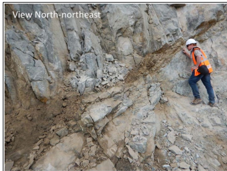
Figure 20: Shallow to intermediate northwest dipping (42 degrees) fault zone, interpreted as a thrust fault. Rory for scale taken after (SRK, 2016).
