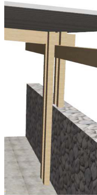
Skin section taken through a part of the building to show column cluster with beams spanning in both directions.
