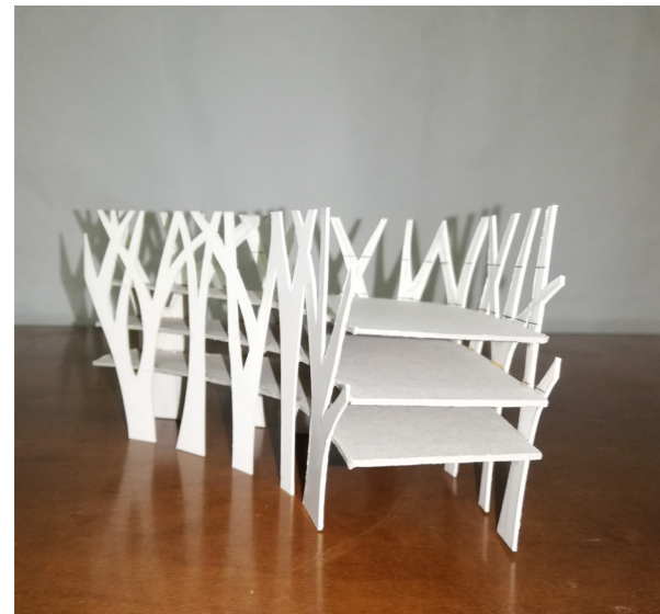
Fig 15: Initial structural system that was investigated, based on the Omotesando building's structure.
