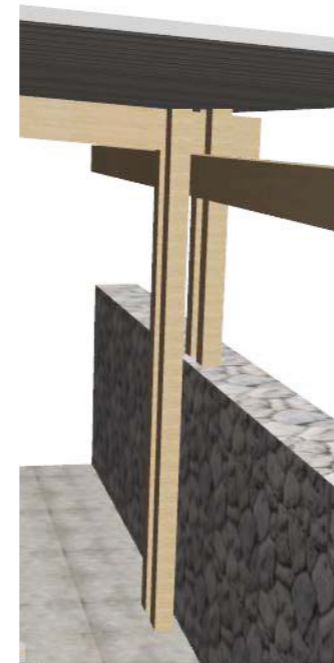
Fig 18: Skin section taken through a part of the building to show column cluster with beams spanning in both directions.
