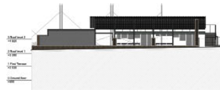
SOUTH WEST ELEVATION |Camping platform Scale 1:100
