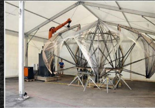
FIG 1: Robot arm using the frame to fabricate the pavilion (Reichert et al., 2014: 28).
