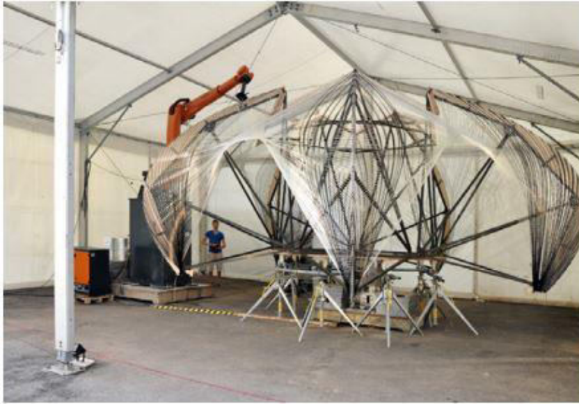
Figure 17: Robot arm using the frame to fabricate the pavilion (Reichert et al., 2014: 28).
