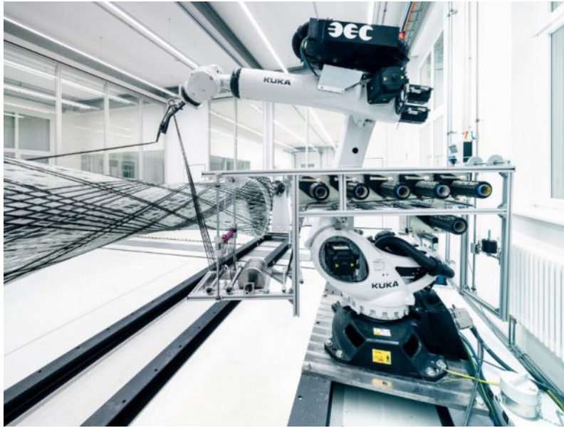
Figure 11: Robot manufacturing the pavilion (Archdaily, 2019, online).
