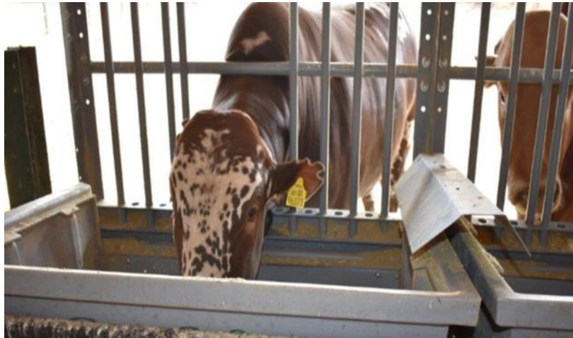
Figure 4.2 An animal feeding from trough suspended on two load cells at a feed intake node (photo taken by Pyoos)
