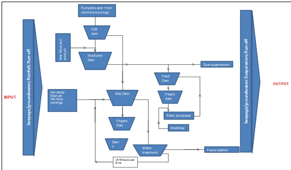
Figure 1.1: Water reticulation at New Vaal Colliery
