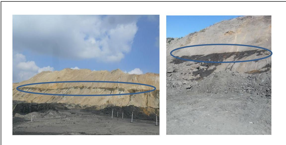
**Figure 2.20: Lateral seepage flow from the perched aquifer**
