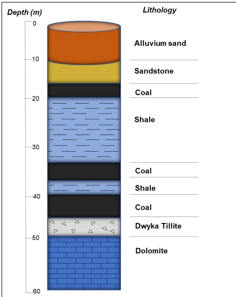
Figure 2.8: Typical borehole log for New Vaal Colliery
