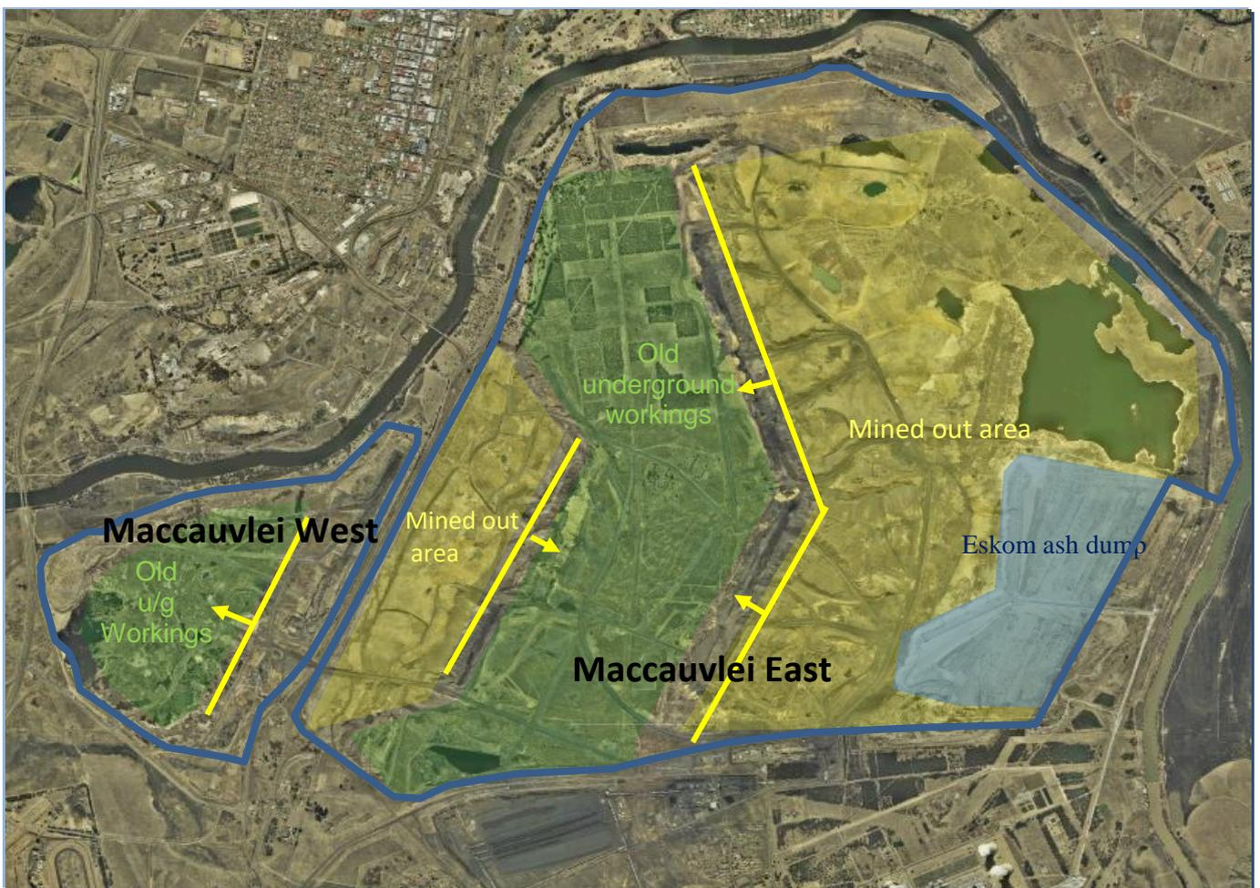
Figure 2.5: Illustration of the old underground mine areas in the Cornelia Coalfield sub-basin
