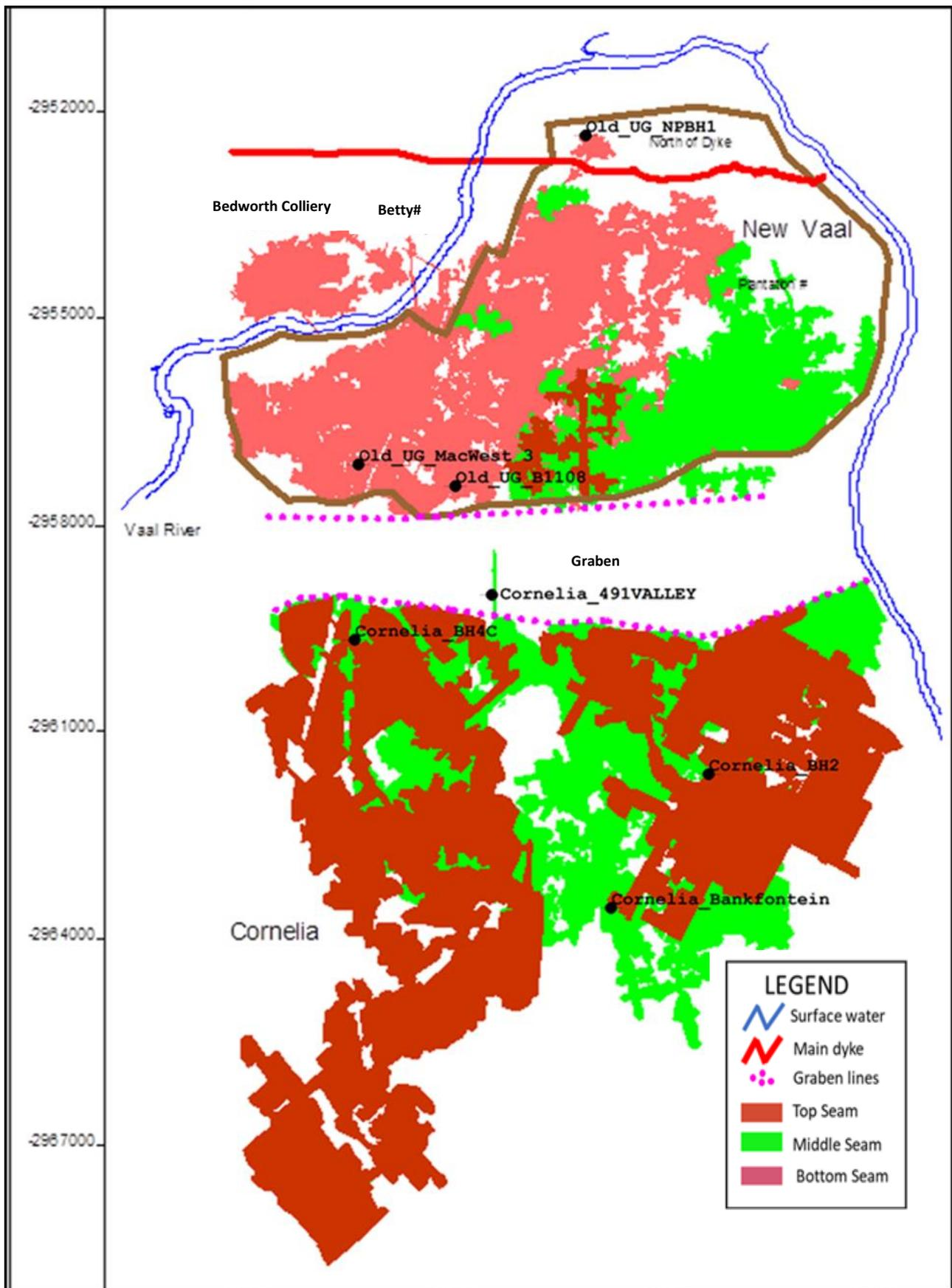
Figure 2.4: Illustration of old underground mine areas in the Cornelia Coalfield sub-basin (Hodgson, 2010)
