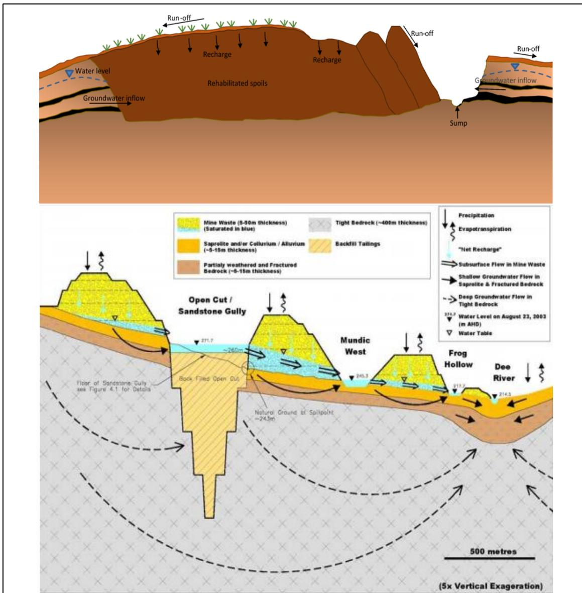
Figure 2.2 Examples of illustrated conceptual groundwater model.
