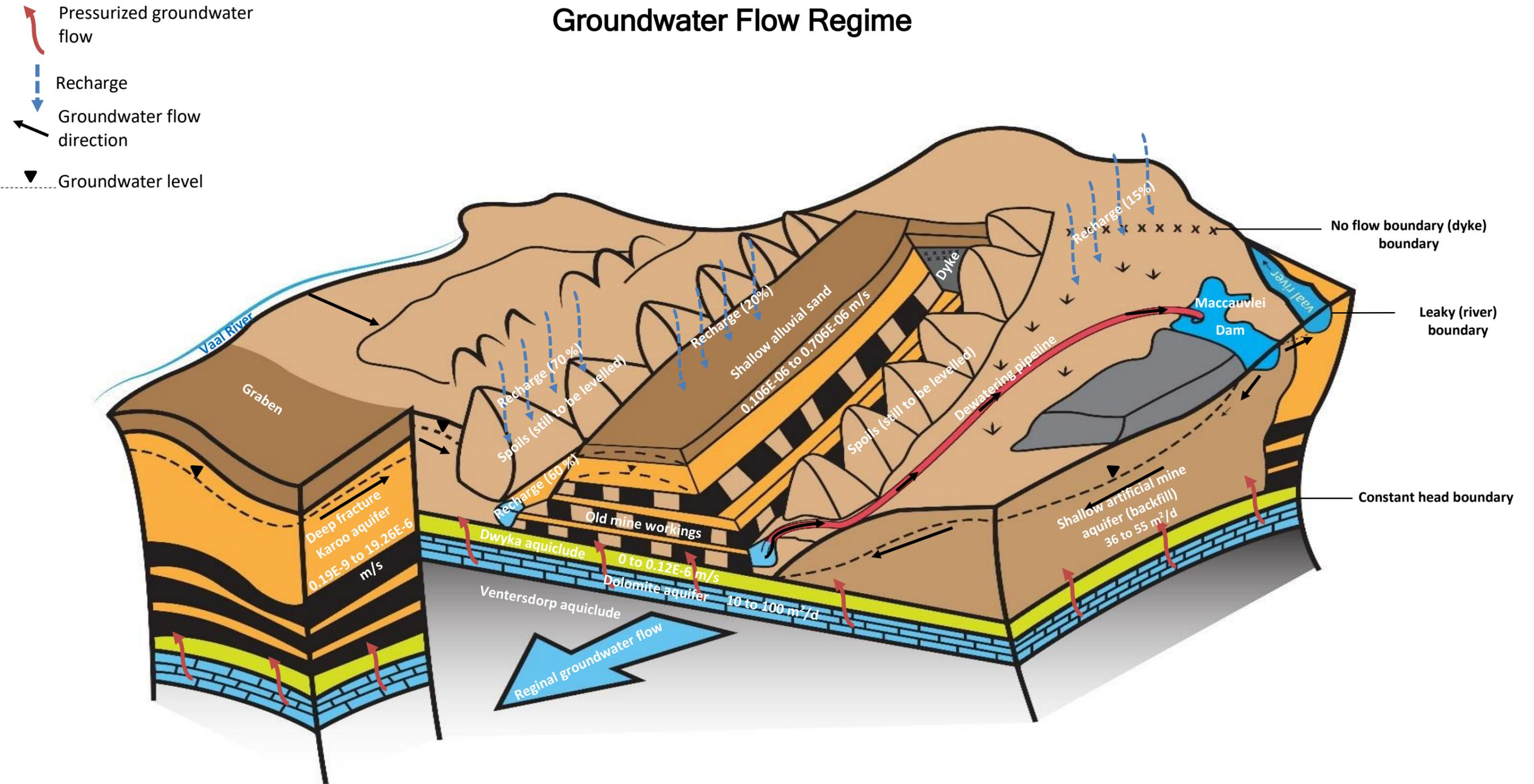
Figure 2.30: Conceptual groundwater flow regime for New Vaal Colliery
