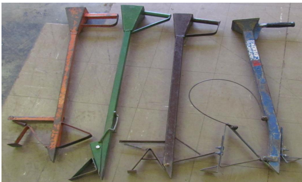
Figure 3.3: Hand planters used to plant maize at the four field trial sites.
