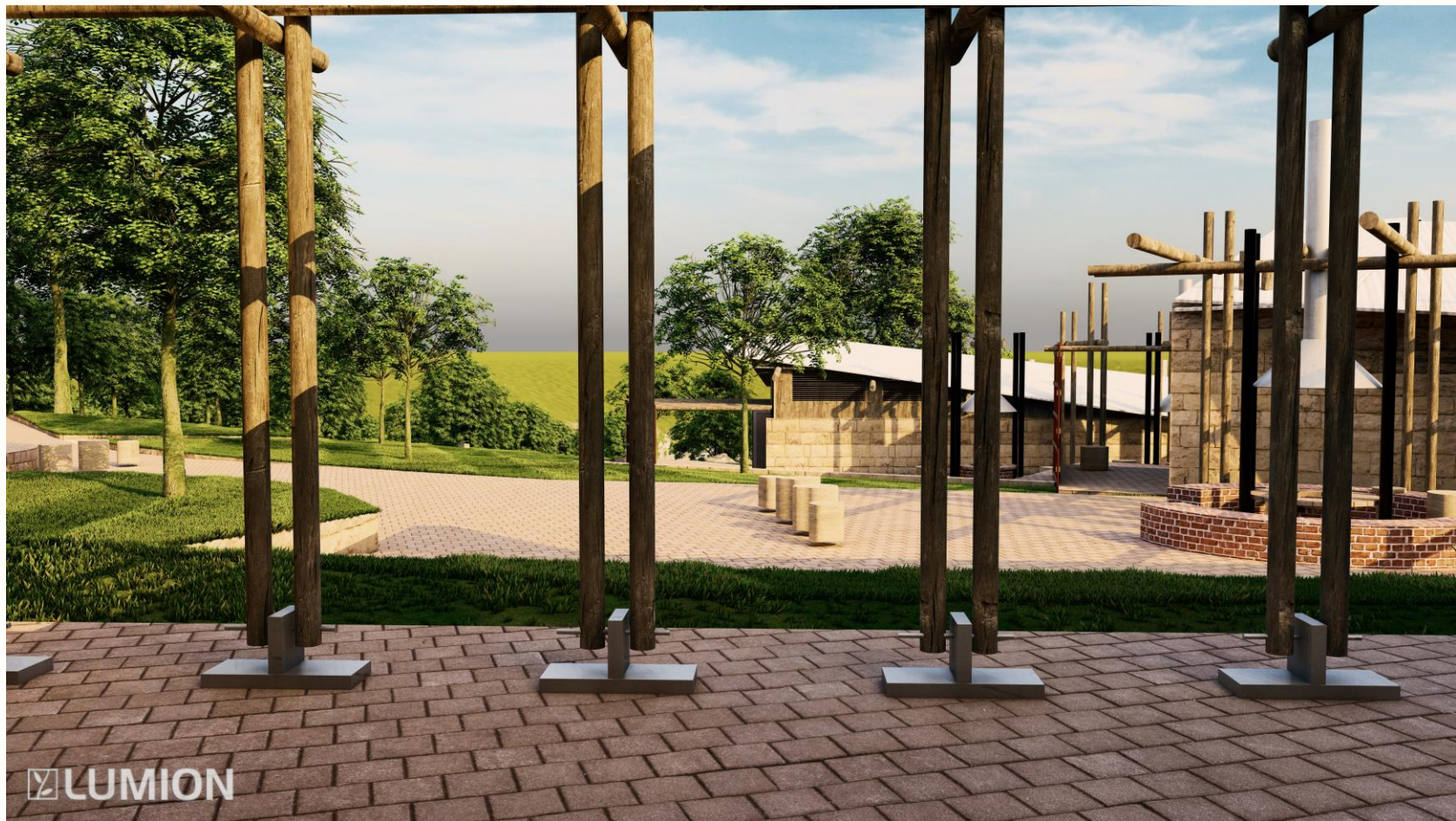
Fig. 178: Detail how to connect outdoor gum poles to the ground for durability (Author 2023)
