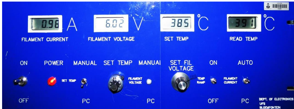
Figure 4.7: The temperature control unit used for controlling the sample temperature in the SAM 600 AES system.
