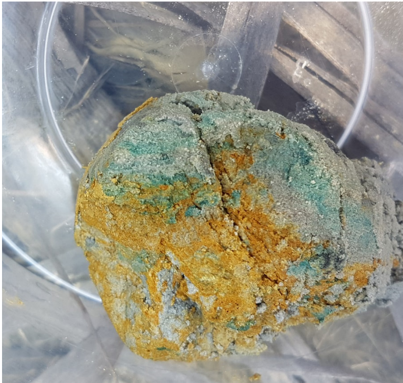
Figure 13: A tailings sample from the Transition Zone showing green and yellow precipitates of hydrated Fe(II)- and Fe(III)-minerals, respectively (August 2015).
