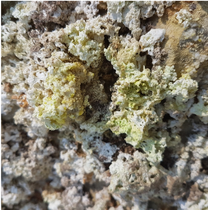
Figure 15: Secondary mineral precipitates from toe seepage. The photo was taken at the location above.
