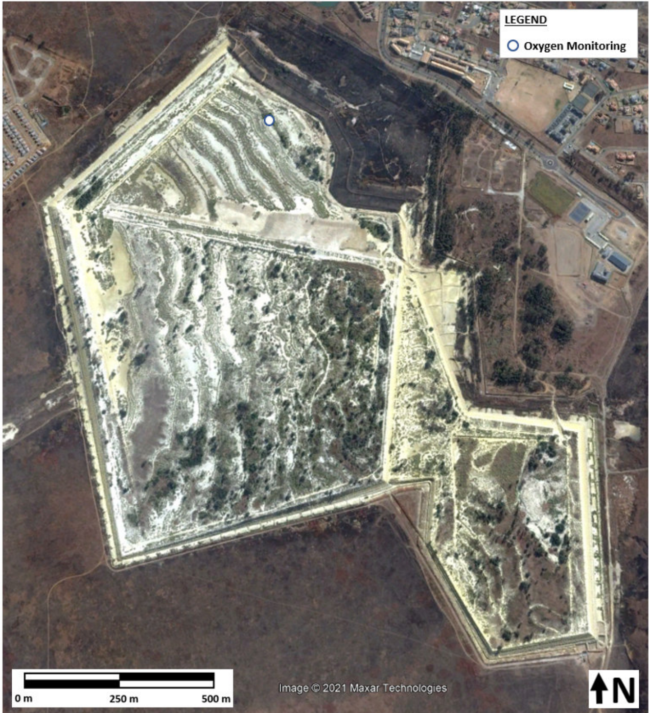
Figure 8: Google image (June 2015) of tailings dam 5L27 and location of oxygen monitoring hole constructed as part of this study. Reclamation of the dam by DRD Gold started in the second half of 2016.
