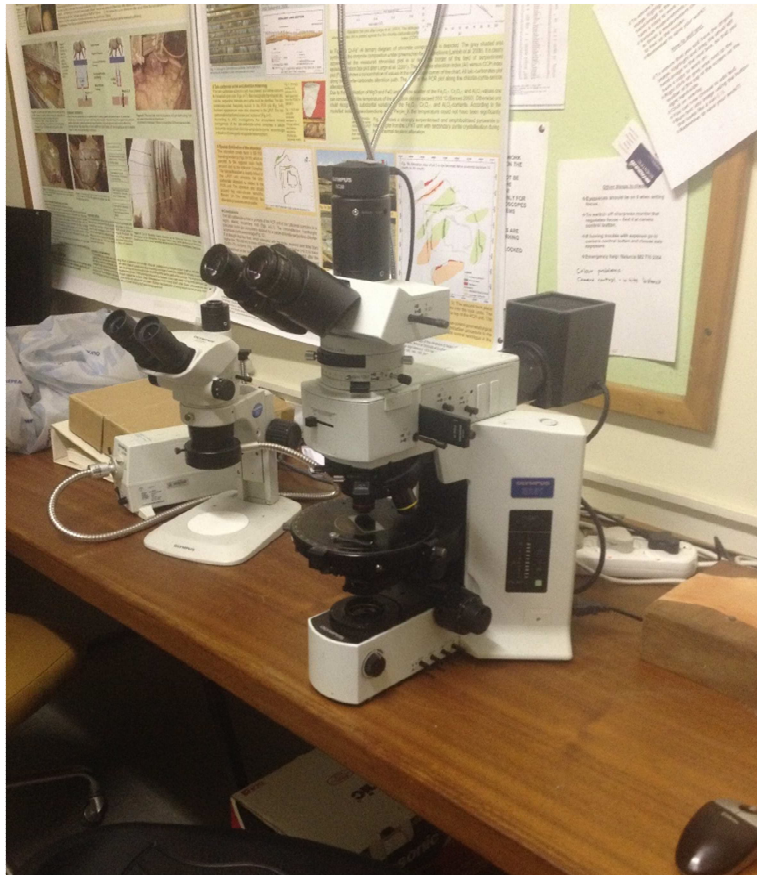
Figure 11: An Olympus BX51 petrographic microscope housed at the Department of Geology, University of the Free State.
