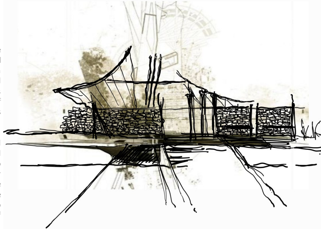
Figure 274 : The structural system consists of stereotomic walls and floating roofs (author, 2022).
