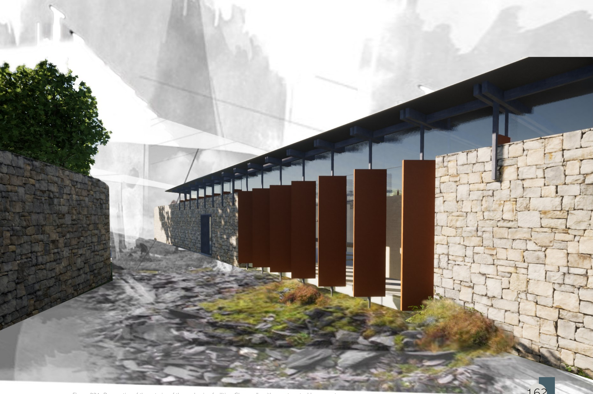
Figure 231: Perspective of the exterior of the packaging facilities. Glass walls with a corten steel louvre system opens up towards the central courtyard (author, 2022).
