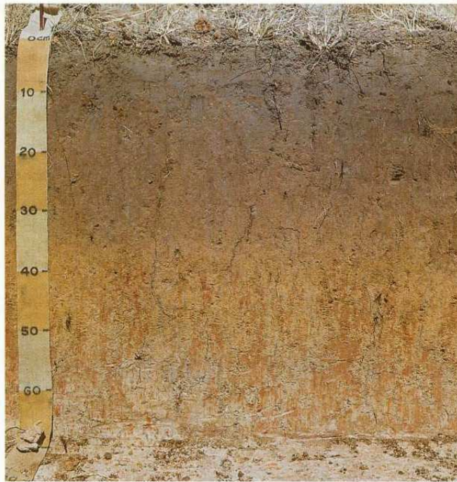
Figure 2.13 Soft plinthic horizon (>35 cm) in a typical Westleigh soil form (Soil Classification Working Group, 1991).
