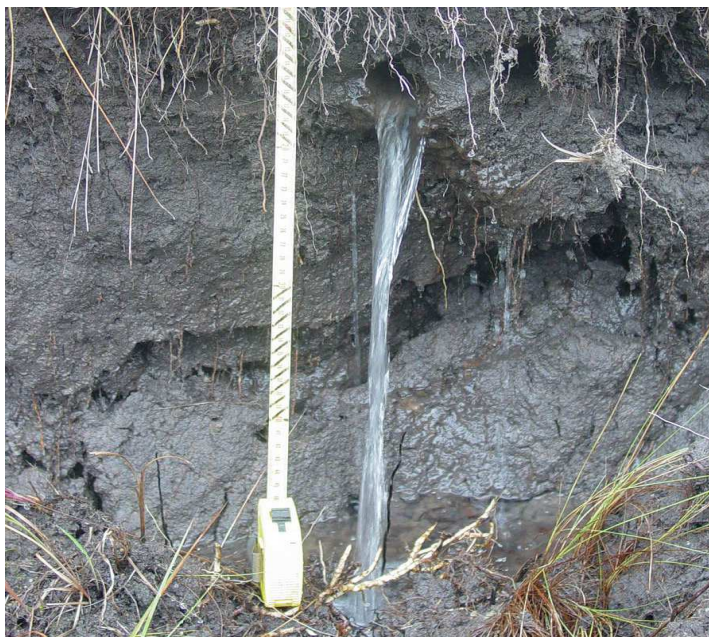
Figure 2.4 Soil pipe outlet (macropore flow) (Photo by Le Roux, 2006).
