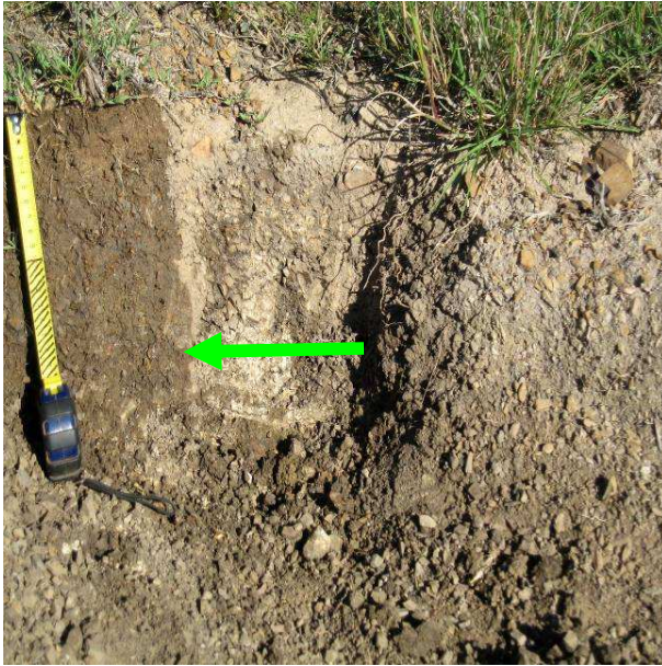
Figure 5.8 Cartref soil form in catchment B4. The E horizon is indicated by arrow.
