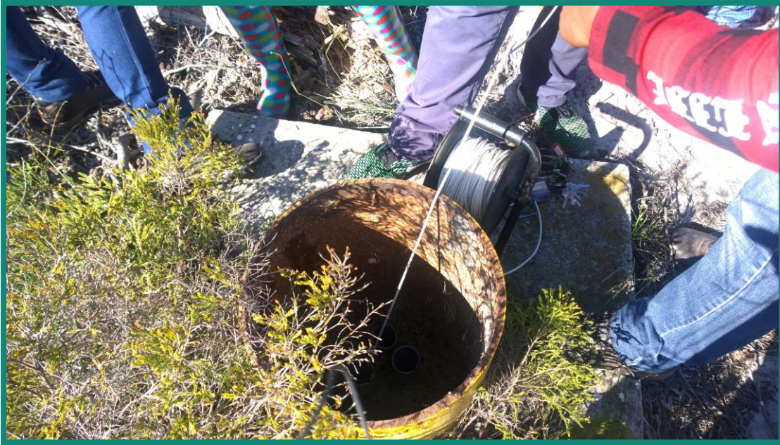
Taking a water level reading at G33333 (22 May 2017)
