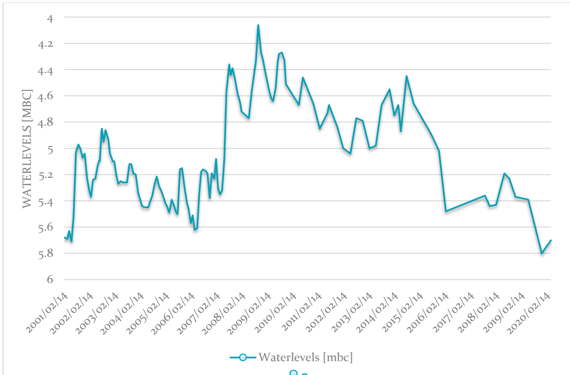
Figure 101: Time series graph of water levels for G33246 with cumulative deviation from mean.
