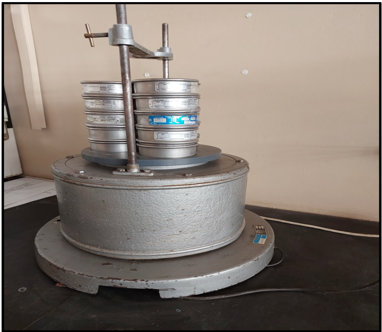
Figure 5.10: Image of horizontal vibrating sieve shaker and sieves used.
